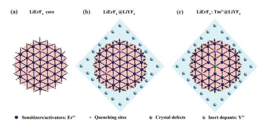
Fig. 3 (a) The energy migration quenching processes in a LiErF<sub>4</sub> UCNP. (b) A typical strategy to reduce the energy migration to surface quenching sites through an inert-shell coating. (c) The approach of simultaneously preventing energy migration quenching processes through introducing  $Tm^{3+}$  ions as energy trapping centers.
