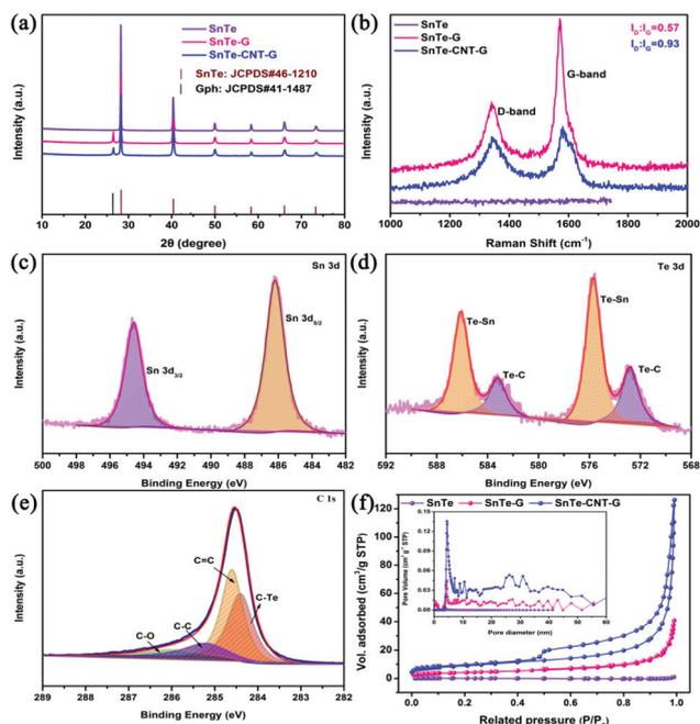
**Fig. 3** (a) XRD patterns of SnTe-CNT-G, SnTe-G and SnTe. (b) Raman spectra of SnTe-CNT-G, SnTe-G and SnTe. Core-level XPS spectra of Sn 3d (c), Te 3d (d) and C 1s (e). (f)  $N_2$  adsorption and desorption isotherm curves of all samples, where the inset shows the pore-size distribution.
