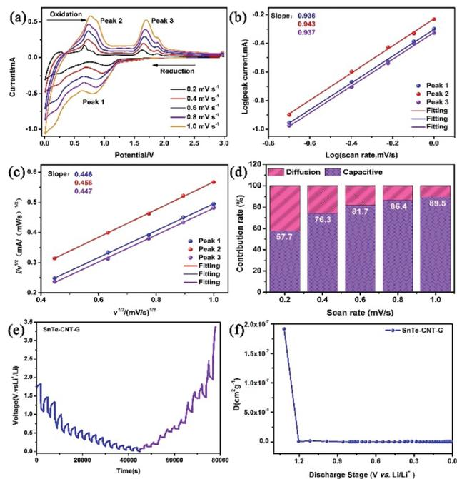
**Fig. 5** (a) CV curves obtained at different scan rates. (b) The corresponding  $\log(i)$  versus  $\log(v)$  plots and (c) the corresponding  $i/v^{1/2}$  versus  $v^{1/2}$  plots of the SnTe-CNT-G electrodes. (d) The normalized ratio of the capacitive- and diffusion-controlled contributions at different scan rates. GITT curves of the SnTe-CNT-G electrode (e) and their  $\text{Li}^+$  diffusion coefficient for the initial discharge states (f).
