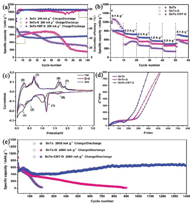
**Fig. 4** (a) Cycling performance and coulombic efficiency of the three samples at  $200 \text{ mA g}^{-1}$ . (b) Rate performance of all samples. (c) CV curves of the SnTe-CNT-G anodes at  $0.2 \text{ mV s}^{-1}$ . (d) Nyquist plots of all electrodes before cycling. (e) Cycling performance at  $2000 \text{ mA g}^{-1}$ .
