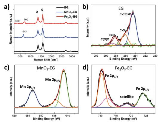
Fig. 3 (a) Raman spectrum of EG, MnO<sub>2</sub>-EG and Fe<sub>2</sub>O<sub>3</sub>-EG composites, and XPS spectrum of (b) C 1s, (c) Mn 2p, and (d) Fe 2p observed in bare EG, MnO2-EG, and Fe2O3-EG composites.
