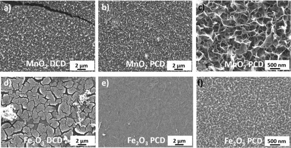
Fig. 2 SEM images of the MnO<sub>2</sub> thin film coated on the EG pattern by (a) direct current deposition (DCD mode, t = 20 min) and (b and c) pulse current deposition methods (PCD mode, t = 40 min); SEM images of the Fe<sub>2</sub>O<sub>3</sub> thin film coated on the EG pattern by (d) direct current deposition (DCD mode, t = 40 min) and (e and f) pulse current deposition methods (PCD mode, t = 80 min).
