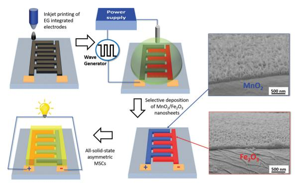
Fig. 1 Schematic illustration of the electrochemical deposition process for Fe<sub>2</sub>O<sub>3</sub> and MnO<sub>2</sub> based inkjet-printed graphene A-MSCs (inset, crosssection SEM images of Fe<sub>2</sub>O<sub>3</sub> and MnO<sub>2</sub> nanoflakes).
