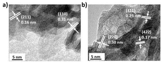
Fig. 4 High magnification TEM images of (a) MnO<sub>2</sub> and (b) Fe<sub>2</sub>O<sub>3</sub> nanoflakes
