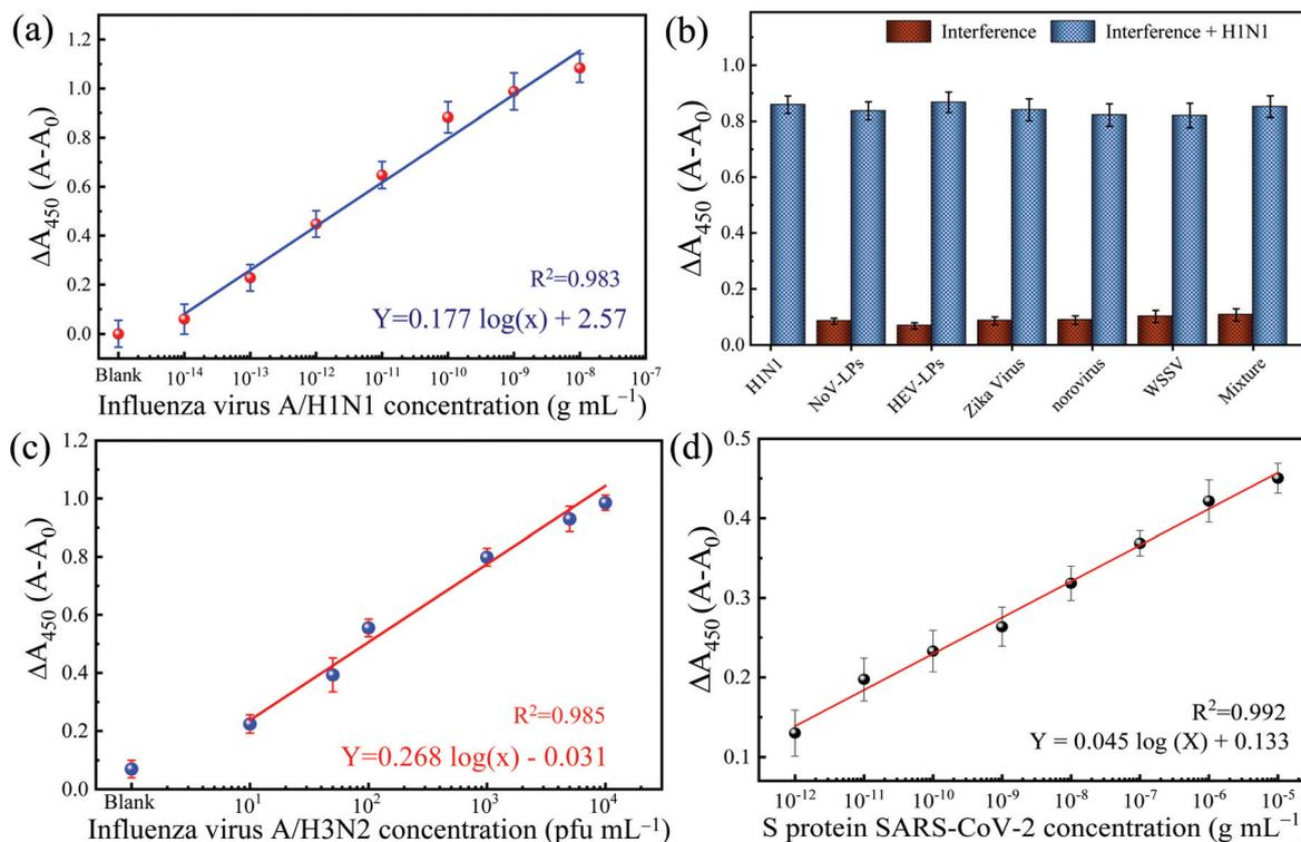
**Fig. 4** (a) The calibration line for the detection of IV/A/H1N1 by TMB-NPs@PLGA based colorimetric detection in the PBS system; (b) the selectivity test in the presence of interferences. The calibration curve obtained using the clinically isolated IV/A/H3N2 (c) and recombinant spike protein of SARS-CoV-2 (d).  $A_0$  indicates the absorbance of a blank sample. The error bars represent the standard deviation of the three measurements.
