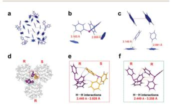
Fig. 4 (a) The interactions of  $Ag_{70}$ -TPP surface ligands; (b) the intramolecular  $C-H\cdots\pi$  interaction; (c) the  $C-H\cdots\pi$  interaction and  $\pi\cdots\pi$ stacking; (d) interaction of adjacent clusters in the lattice; (e)  $H \cdots H$ interactions of the cluster with opposite chirality; (f) H...H interactions of the cluster with the same chirality.
