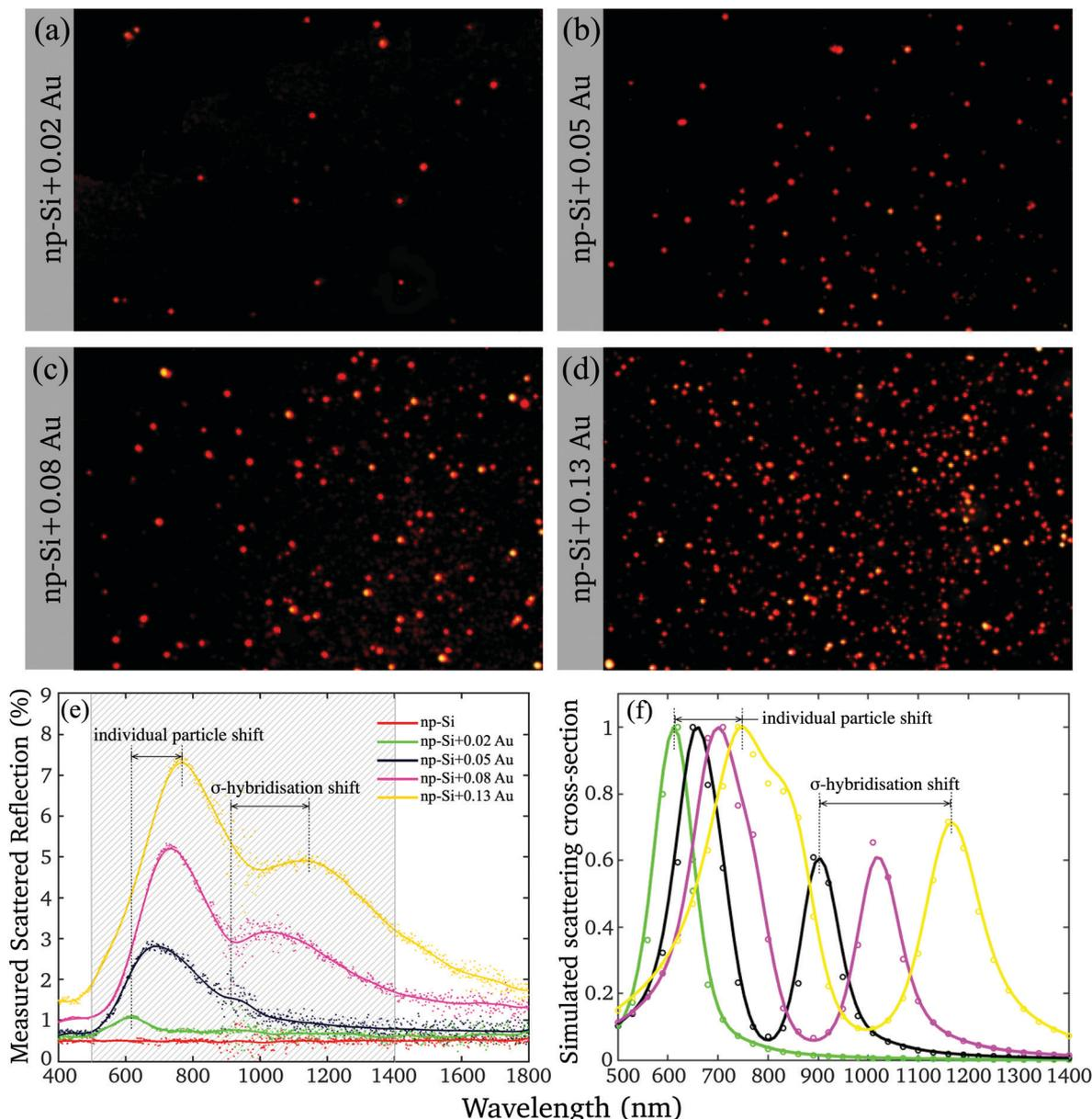
Fig. 2 (a–d) Dark Field Microscope (DFM) images of the four samples with different Au volume fractions; (e) measured scattered reflection of np-Si samples without and with different volume fraction of Au; (f) simulated scattering cross-section (normalised) for the fitting parameters listed in Table 2.
