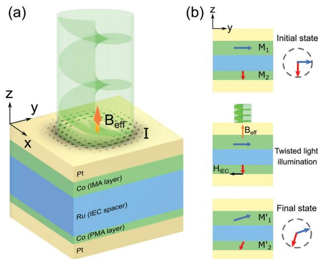
**Fig. 5** The proposed schematic diagram summarizing the mechanism involving the twisted light's modification to the MA of the IEC heterojunction. (a) The 3D model of a twisted light beam illuminating the sample. The circular current  $I$ , which is triggered by the twisted light, induces an effective field  $B_{\text{eff}}$ . (b) Step-by-step figures describing the evolution of the spin configuration modified by the twisted light.
