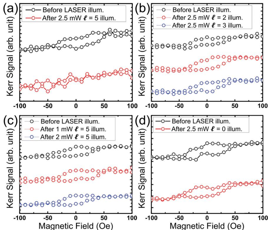
**Fig. 3** A series of Kerr signal comparisons between before and after laser illumination of the sample. The different parameters are shown as follows. (a) The OAM laser ( $\ell = 5$ ) with a power of 2.5 mW could change the sample from ferromagnetic into paramagnetic. (b) Lasers of different OAM ( $\ell = 2, \ell = 3$ ) with a fixed power of 2.5 mW. (c) Fixed OAM laser ( $\ell = 5$ ) with lower power. (d) A fundamental laser with linear polarization.
