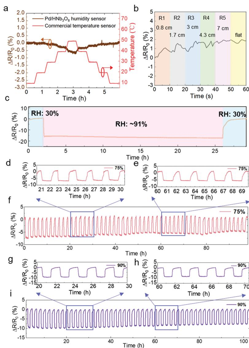
Fig. 4 (a) Temperature dependent test of a 1% Pd/HNb<sub>3</sub>O<sub>8</sub> humidity sensor under temperature variations from 10 °C to 50 °C. (b) Real-time bending result of a 1% Pd/HNb<sub>3</sub>O<sub>8</sub> humidity sensor under various bending radii. (c) 24 h stability test of a 1% Pd/HNb<sub>3</sub>O<sub>8</sub> humidity sensor under 90% RH. Long-term stability measurements (50 cycles) under (d–f) 75% RH and (g–i) 90% RH.
