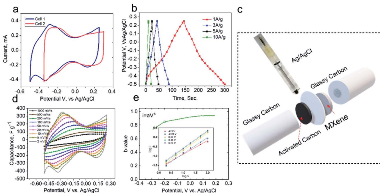
Fig. 2 (a) CV curves of Mo<sub>1.33</sub>C MXene at 20 mV s<sup>-1</sup> using stainless steel (cell 1) and glass carbon (cell 2) as current collectors, respectively; (b) charge/discharge and (d) CV curves of Mo<sub>1.33</sub>C MXene at different current densities and scan rates; and (c) schematic illustration of the three-electrode setup; and (e) *b*-values at different potentials ( $i = av^b$ ).
