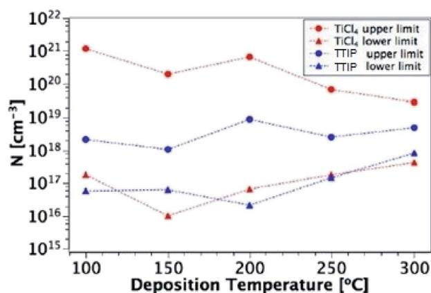
Fig. 12 Upper and lower limits of  $N$  for films deposited from TiCl<sub>4</sub> and TTIP over the temperature range 100–300 °C.
