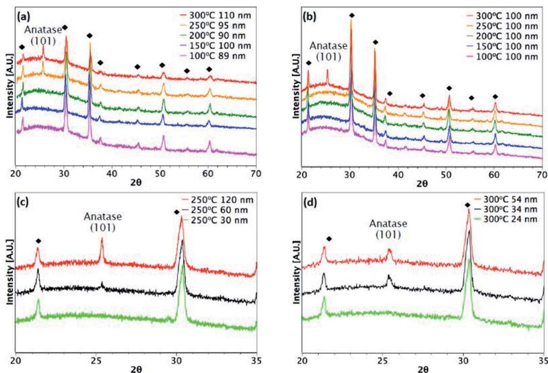
Fig. 4 XRD patterns for  $\text{TiO}_2$  films deposited on ITO. Black diamonds indicate peaks from the underlying ITO. Films deposited at different temperatures from (a)  $\text{TiCl}_4$  and (b) TTIP. Different film thicknesses deposited from (c)  $\text{TiCl}_4$  at 250 °C and (d) TTIP at 300 °C.
