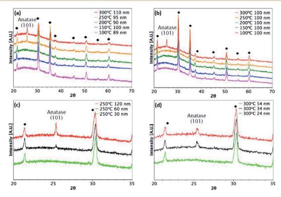
Fig. 4 XRD patterns for  $TiO_2$  films deposited on ITO. Black diamonds indicate peaks from the underlying ITO. Films deposited at different temperatures from (a)  $TiCl_4$  and (b) TTIP. Different film thicknesses deposited from (c)  $TiCl_4$  at 250 °C and (d) TTIP at 300 °C.
