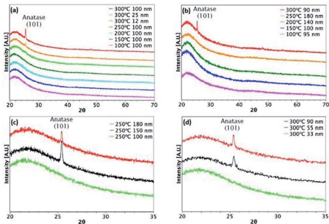
Fig. 3 XRD patterns for  $\text{TiO}_2$  films deposited on glass. Films deposited at different temperatures from (a)  $\text{TiCl}_4$  and (b) TTIP. Different film thicknesses deposited at (c) 250 °C from  $\text{TiCl}_4$  and (d) 300 °C from TTIP.
