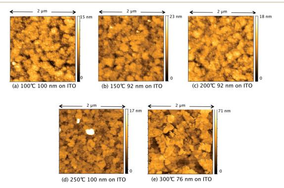
Fig. 7 AFM images of TiO<sub>2</sub> films deposited at different temperatures on ITO from TTIP. Film thicknesses and deposition temperatures presented under each of the images, labelled (a)-(e).
