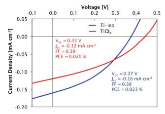
Fig. 13 Current density–voltage curves for glass/ITO/TiO<sub>2</sub>/P3HT/  $MoO_3$ /Ag cells under simulated AM1.5 solar illumination (100 mW cm<sup>-2</sup>). TiO<sub>2</sub> films deposited from TiCl<sub>4</sub> and TTIP.
