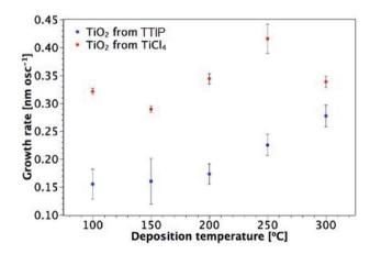
Fig. 2  $\,$  Growth rate of TiO $_2$  films from TiCl $_4$  and TTIP as a function of deposition temperature.
