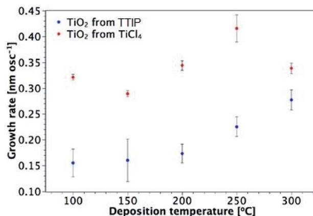
Fig. 2 Growth rate of TiO<sub>2</sub> films from TiCl<sub>4</sub> and TTIP as a function of deposition temperature.
