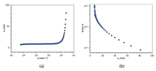
Fig. 11 Resulting (a)  $x_e$  vs.  $\omega$  and (b) N vs.  $x_e$  plots for the film deposited from TTIP
