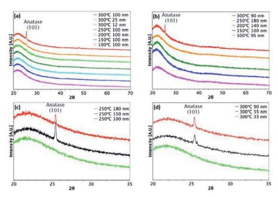
Fig. 3 XRD patterns for  $TiO_2$  films deposited on glass. Films deposited at different temperatures from (a)  $TiCl_4$  and (b) TTIP. Different film thicknesses deposited at (c) 250 °C from  $TiCl_4$  and (d) 300 °C from TTIP.
