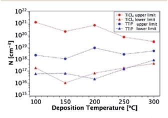
Fig. 12 Upper and lower limits of N for films deposited from TiCl<sub>4</sub> and TTIP over the temperature range 100-300 °C.
