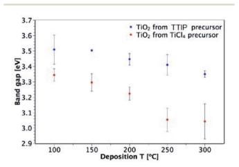
Fig. 9 Dependence of TiO<sub>2</sub> band gap on precursor and deposition temperature (for 50-150 nm-thick films deposited on glass).
