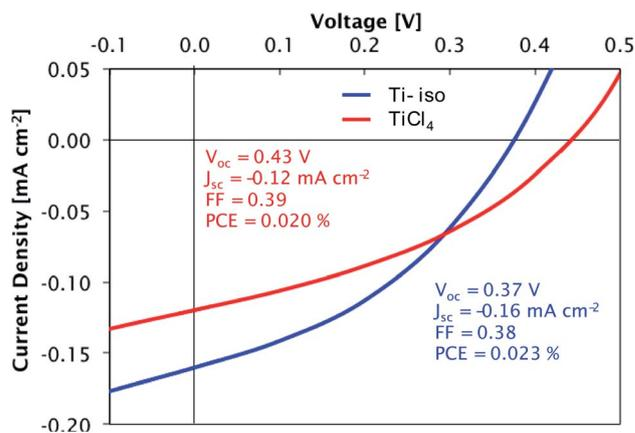
Fig. 13 Current density–voltage curves for glass/ITO/TiO<sub>2</sub>/P3HT/MoO<sub>3</sub>/Ag cells under simulated AM1.5 solar illumination (100 mW cm<sup>-2</sup>). TiO<sub>2</sub> films deposited from TiCl<sub>4</sub> and TTIP.
