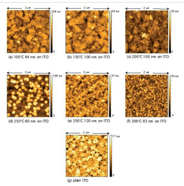
Fig. 5 AFM images of  $TiO_2$  films deposited at different temperatures on ITO from  $TiCl_4$ . Film thicknesses and deposition temperatures presented under each of the images, labelled (a)–(g). ITO roughness:  $2.9 \pm 0.3$  nm.
