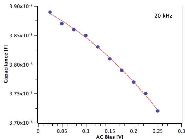
Fig. 10 Capacitance vs. AC bias at 20 kHz for a TiO<sub>2</sub> film deposited from TTIP at 200 °C.
