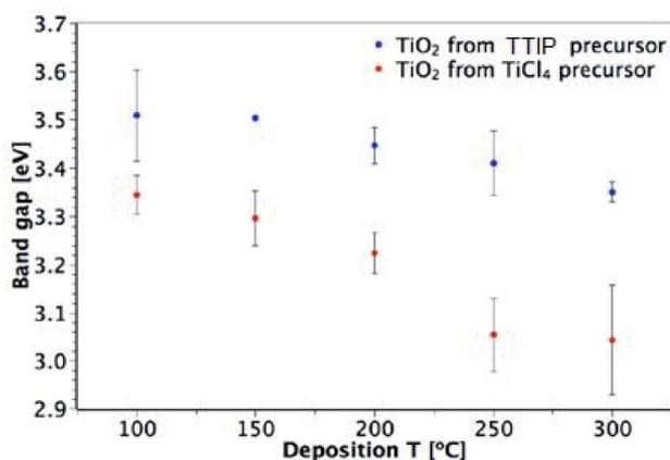
Fig. 9 Dependence of TiO<sub>2</sub> band gap on precursor and deposition temperature (for 50–150 nm-thick films deposited on glass).
