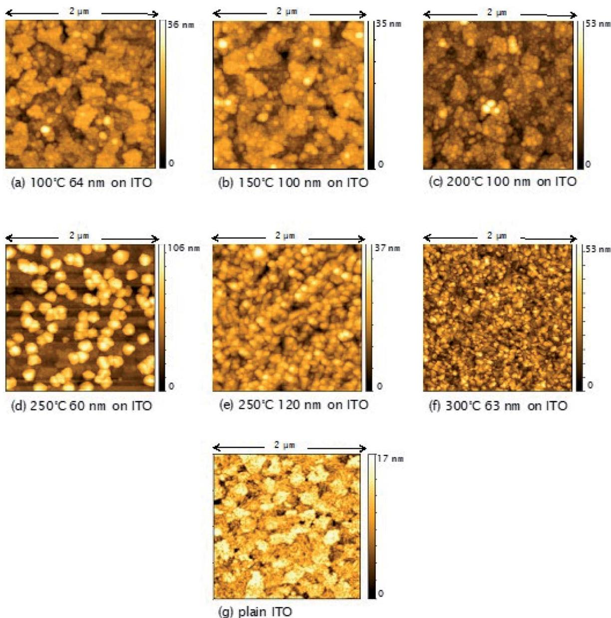
Fig. 5 AFM images of  $\text{TiO}_2$  films deposited at different temperatures on ITO from  $\text{TiCl}_4$ . Film thicknesses and deposition temperatures presented under each of the images, labelled (a)–(g). ITO roughness:  $2.9 \pm 0.3$  nm.
