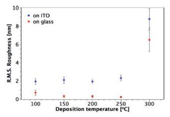
Fig. 8 Plot showing the variation of R.M.S. roughness with deposition temperature for TiO<sub>2</sub> films deposited from TTIP on glass and ITO. Film thicknesses are indicated in Fig. 7 and S3.†
