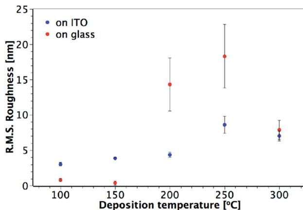
Fig. 6 Plot showing the variation of R.M.S. roughness with deposition temperature for TiO<sub>2</sub> films deposited from TiCl<sub>4</sub> on glass and ITO. Film thicknesses are indicated in Fig. 5 and S2.†
