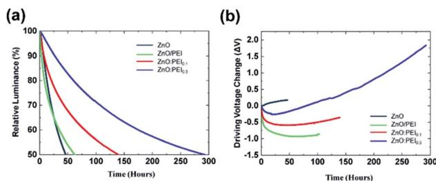
Fig. 3 Relative luminance (a) and changes in driving voltage (b) vs. time trends of the QDLEDs with the different ETLs under 20 mA cm<sup>-2</sup> constant current driving conditions.
