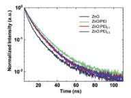
Fig. 2 TRPL characteristics of the QDs on ZnO, ZnO/PEI, ZnO:PEI $_{0.1}$  and ZnO:PEI $_{0.3}$ .
