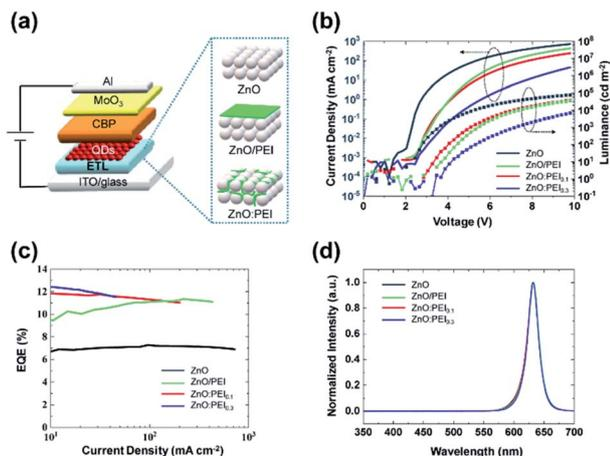
Fig. 1 (a) Schematic diagram showing the general structure of the QDLEDs and the different ETLs investigated in this work. (b)  $J$ - $V$ - $L$  characteristics, (c) EQE, and (d) electroluminescence spectra of the QDLEDs.
