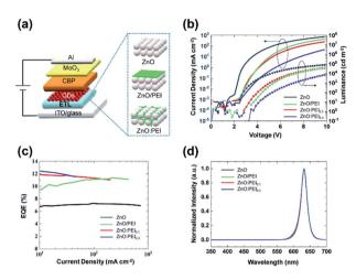
Fig. 1 (a) Schematic diagram showing the general structure of the QDLEDs and the different ETLs investigated in this work. (b) J-V-L characteristics, (c) EQE, and (d) electroluminescence spectra of the QDLEDs.
