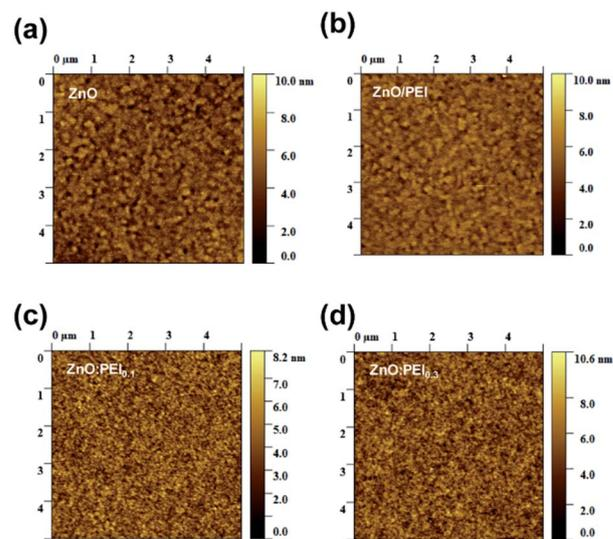
Fig. 4 AFM surface topography images of (a) ZnO, (b) ZnO/PEI, (c) ZnO:PEI<sub>0.1</sub>, and (d) ZnO:PEI<sub>0.3</sub>.
