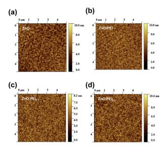
Fig. 4 AFM surface topography images of (a) ZnO, (b) ZnO/PEI, (c) ZnO:PEI $_{0.1}$ , and (d) ZnO:PEI $_{0.3}$ .
