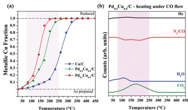
Fig. 1 (a) Temperature dependence of the metallic Cu fraction of  $\text{Pd}_x\text{Cu}_{1-x}/\text{C}$  samples during heating under a CO flow. (b) Mass spectrometry results of major compounds formed during the heating of  $\text{Pd}_{0.5}\text{Cu}_{0.5}/\text{C}$  under a CO flow.
