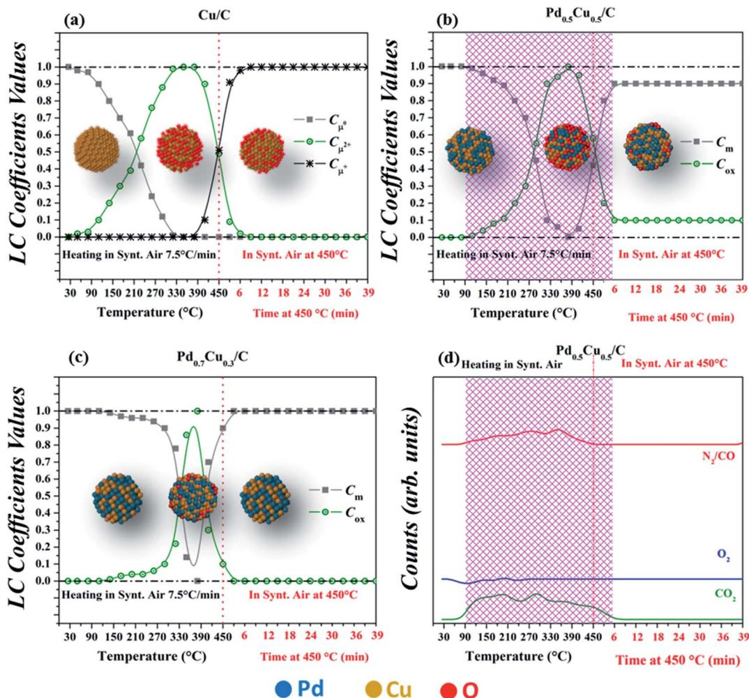
Fig. 4 Oxidation reaction with synthetic air: evolution of the coefficients employed for the linear combination of the XANES spectra of Cu/C (a),  $Pd_{0.5}Cu_{0.5}/C$  (b) and  $Pd_{0.7}Cu_{0.3}/C$  (c) presented as a function of the temperature (during the heating up to 450 °C) and of time (while the samples were kept at 450 °C), and (d) the mass spectrometry counts of major compounds observed during the heating under a synthetic air flow of  $Pd_{0.5}Cu_{0.5}/C$ .
