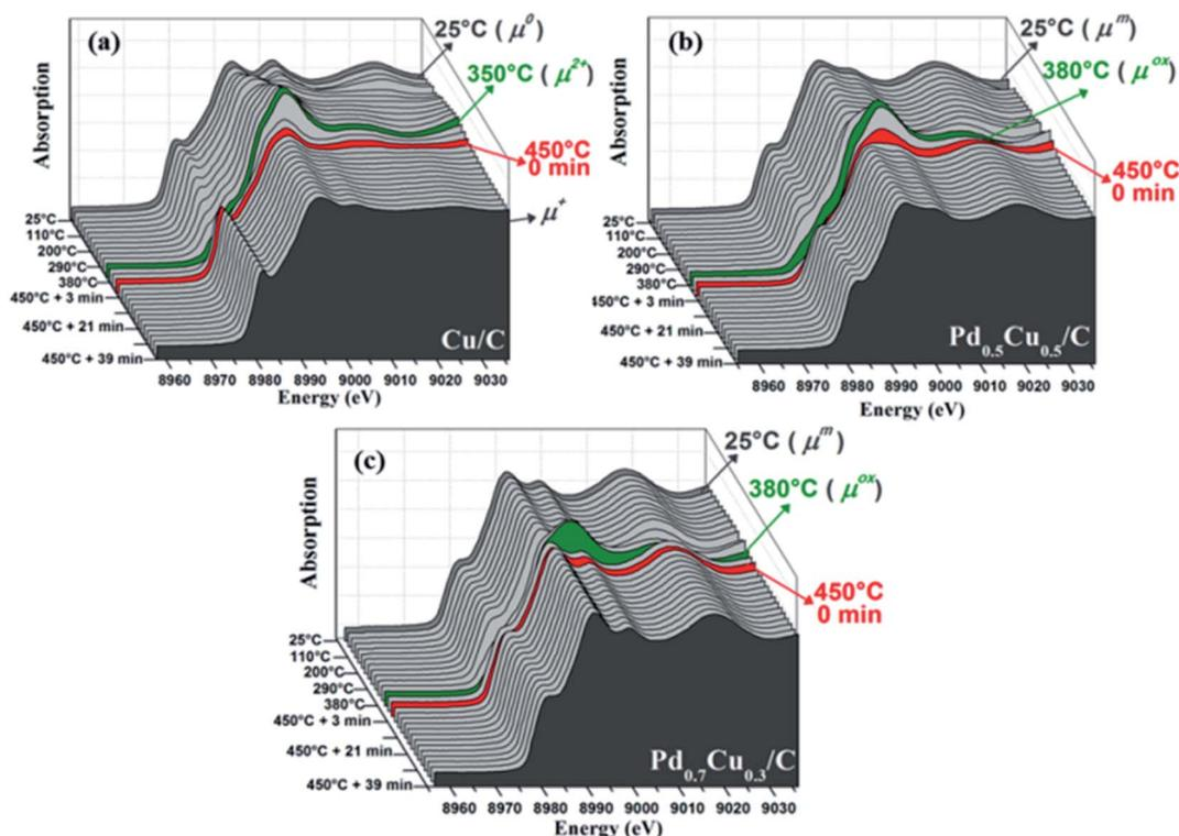
Fig. 3 Oxidation reaction with synthetic air: evolution of the Cu K edge XANES spectra of Cu/C (a), Pd<sub>0.5</sub>Cu<sub>0.5</sub>/C (b) and Pd<sub>0.7</sub>Cu<sub>0.3</sub>/C (c) presented as a function of temperature (during the heating up to 450 °C) and time (while the samples were kept at 450 °C).
