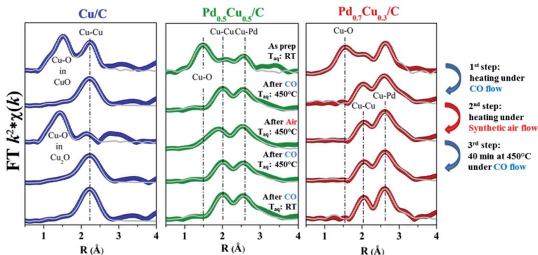
Fig. 2 Cu K edge EXAFS analyses: FT of  $k^2$ -weighted EXAFS signals collected after each step of reaction for all samples. The experiment steps and the acquisition temperatures are indicated in the spectra. The closed circles correspond to the experimental data and the grey continuous lines are the best obtained fits.
