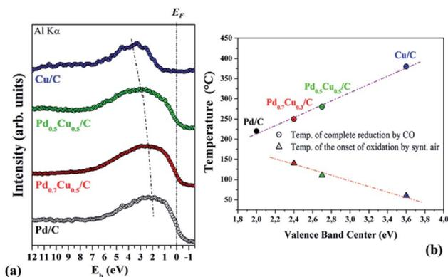
Fig. 5 (a) Valence band photoemission spectra for the as-prepared Cu/C,  $Pd_{0.5}Cu_{0.5}/C$ ,  $Pd_{0.7}Cu_{0.3}/C$  and Pd/C. (b) Relationship between the binding energy of the valence band center of each sample, the temperature for their complete reduction by CO and the onset temperature during oxidation in synthetic air.
