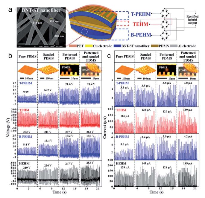
Fig. 6 Modification of surface roughness to improve the electrical output. (a) Schematic of an all-in-one PDMS-PVDF/BNT/ST nanofibre hybrid energy harvester module structure. (b) Output voltage and (c) output current of the PTENG corresponding with the surface roughness of the PDMS layer. Reprinted with permission from ref. 49. Copyright (2020) American Chemical Society.
