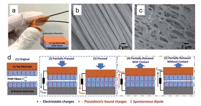
Fig. 5 A PTENG based on aligned electrospun polyvinylidene fluoride (PVDF) fibre mats. (a) Photo and schematic of the PVDF fibre energy harvesting device. SEM image of the bundles of the aligned as-spun fiber (b) and melted at 185 °C (c). (d) Constructive piezoelectric-triboelectric effect in PVDF fibres with aligned electrical polarization. Reproduced with permission.<sup>47</sup> Copyright 2020, John Wiley and Sons.
