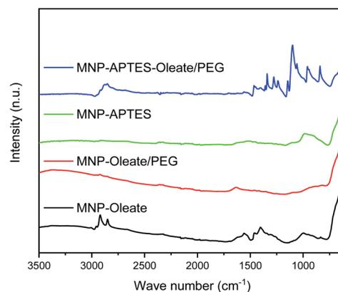
Fig. 1 ATR-IR spectra of dried differently coated MNPs.
