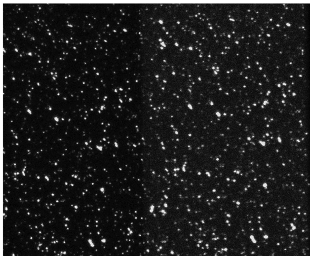
Fig. 7 Typical fluorescence images obtained with the exposure of 70 ms of nanoparticles/nanothermometers adhered to a glass surface in water. Both spectral bands are shown: 530 nm (right image) and 580 nm (left image). The vertical scale is 65 microns.
