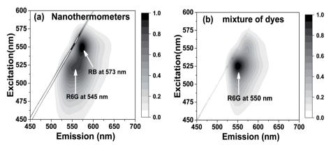
Fig. 2 Emission and excitation matrices of (a) nanothermometers and (b) free dyes in water in the same proportions as those inside the nanothermometers but heavily dissolved (0.10  $\mu$ M R6G and 0.09  $\mu$ M RB, the proportion is similar to that inside the nanothermometers). Both matrices are recorded at room temperature.
