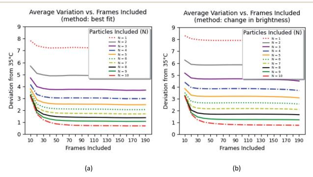
Fig. 8 The average error of measurements of 35 °C using 1–10 nanothermometers while measuring the fluorescence signal between 700 ms (10 frames) and 14 s (200 frames). Two different methods of background subtraction were used: (a) the best fit using a polynomial function and (b) average background calculated within the region of interest (around each particle).
