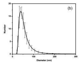
Fig. 1 (a) A representative TEM image (scale bar is 50 nm). A  $74 \times 74$  nm<sup>2</sup> inset shows the mesoporous structure of the nanothermometers. (b) The particle size distribution obtained from DLS measurements. The error bar corresponds to the standard deviation obtained from five measurements.
