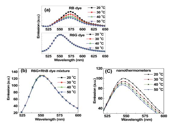
Fig. 3 Fluorescence spectra upon excitation at 488 nm at different temperatures for (a)  $0.1~\mu M$  R6G dye,  $0.09~\mu M$  RB dye, (b) a mix of  $0.1~\mu M$  R6G and  $0.09~\mu M$  RB dyes, and (c) nanothermometers.
