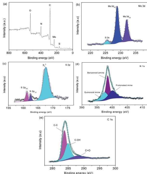
Fig. 6 (a) XPS survey spectrum, and (b) Mo 3d, (c) S 2p, (d) N 1s, and (e) C 2p spectra of MoS<sub>2</sub>@C@PANI.
