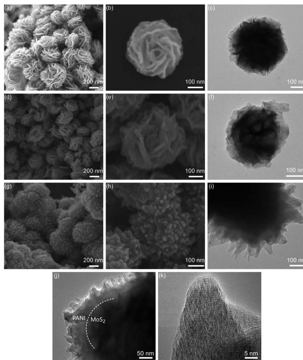
Fig. 2 SEM images of (a and b) flower-shaped  $\text{MoS}_2$ , (d and e)  $\text{MoS}_2\text{@C}$ , and (g and h)  $\text{MoS}_2\text{@C@PANI}$ . TEM images of the (c) bare  $\text{MoS}_2$ , (f)  $\text{MoS}_2\text{@C}$  composite and (i)  $\text{MoS}_2\text{@C@PANI}$ . (j and k) HRTEM images of  $\text{MoS}_2\text{@C@PANI}$ . The dashed line in j indicates the boundary between  $\text{MoS}_2$  and PANI.
