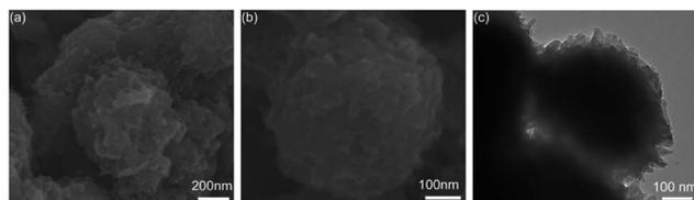
Fig. 10 (a and b) SEM and (c) TEM images of MoS<sub>2</sub>@C@PANI after 100 cycles at 0.1 A g<sup>-1</sup>.
