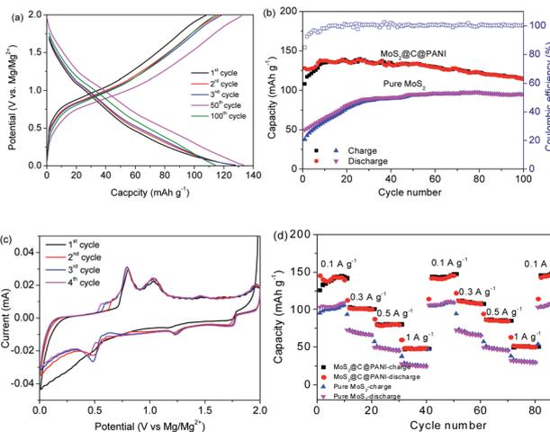
Fig. 7 (a) Charge-discharge curves of MoS<sub>2</sub>@C@PANI at 0.1 A g<sup>-1</sup>. (b) Capacities and coulombic efficiency. (c) CV curves cycled at 0.1 mA s<sup>-1</sup>. (d) Rate-performance.
