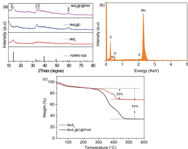
Fig. 4 (a) XRD patterns of MoS<sub>2</sub>, MoS<sub>2</sub>@C, and MoS<sub>2</sub>@C@PANI. (b) EDS spectrum of MoS<sub>2</sub>@C@PANI. (c) TGA curve of bare MoS<sub>2</sub> and MoS<sub>2</sub>@C@PANI.
