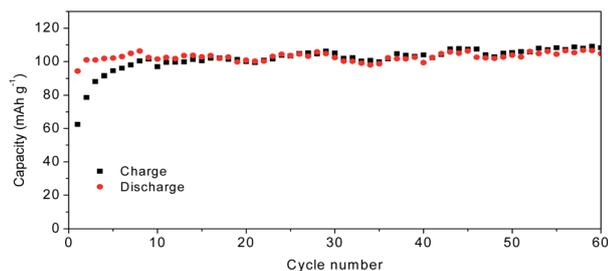
Fig. 8 Capacity of the MoS<sub>2</sub>@C@PANI cathode cycled at 0.1 A g<sup>-1</sup> at -5 °C.
