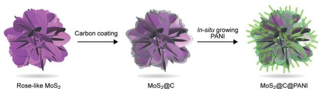
Fig. 1 Illustration of the preparation of ternary  $\text{MoS}_2\text{@C@PANI}$ .
