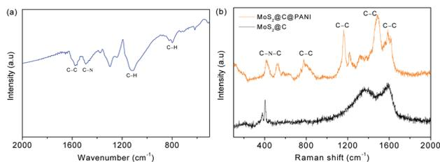
Fig. 5 (a) FTIR spectrum of MoS<sub>2</sub>@C@PANI. (b) Raman spectra of bare MoS<sub>2</sub> and the MoS<sub>2</sub>@C@PANI composite.
