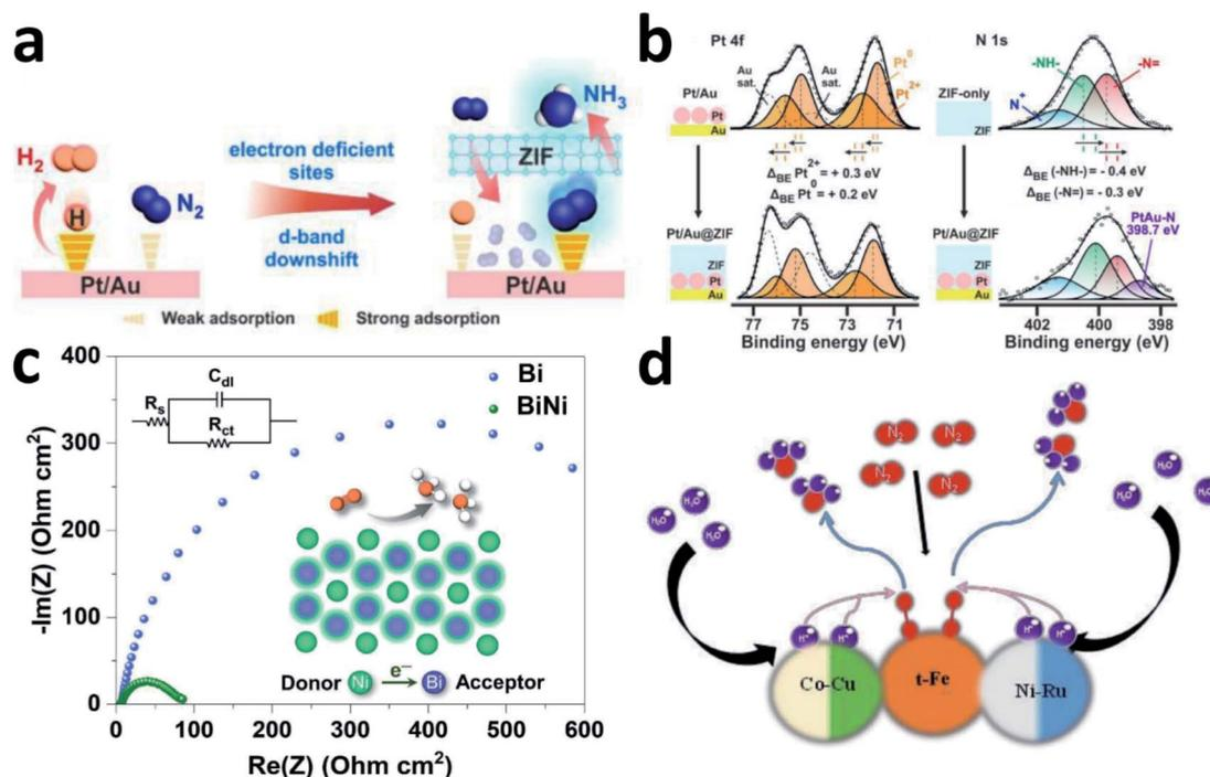
Fig. 7 (a) Schematic depicting the functions of Pt/Au@ZIF. (b) XPS investigations on the Pt/Au@ZIF platform. Copyright 2020, Wiley-VCH.<sup>36</sup> (c) EIS spectra of Bi and BiNi. Copyright 2020, Wiley-VCH.<sup>147</sup> (d) Schematic illustration of a possible mechanism of RuFeCoNiCu NPs. Copyright 2020, Wiley-VCH.<sup>148</sup>
