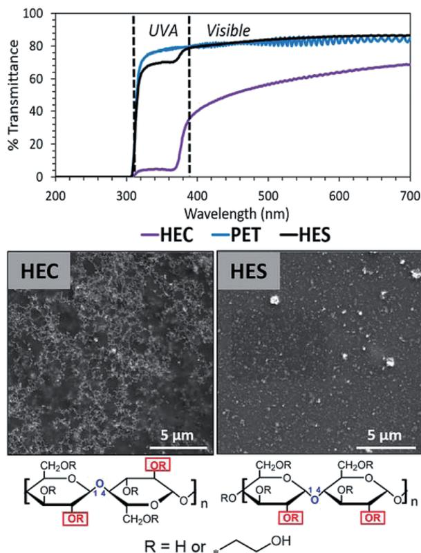
Fig. 8 Cluster and network structures of zinc oxide nanoparticles in hydroxyethyl starch and hydroxyethyl cellulose matrices. Only network structures promote UV-blocking. This figure has been adapted from ref. 164 with permission from ACS Publications, 2019.
