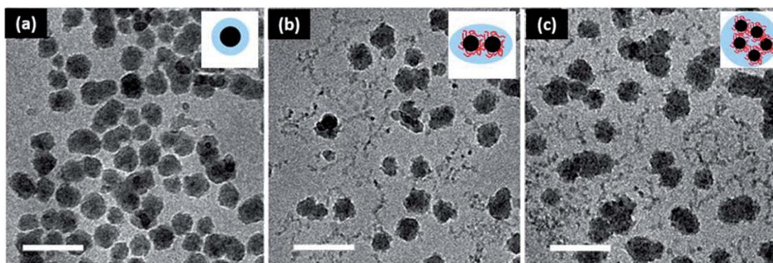
Fig. 4 Silica cluster formation with hydroxyethyl cellulose loading for drug delivery applications. (a) 0.1% w/v, (b) 0.5% w/v, and (c) 1% w/v hydroxyethyl cellulose. Scale bar is 100 nm. This figure has been adapted from ref. 176 with permission from the Royal Society of Chemistry, 2018.
