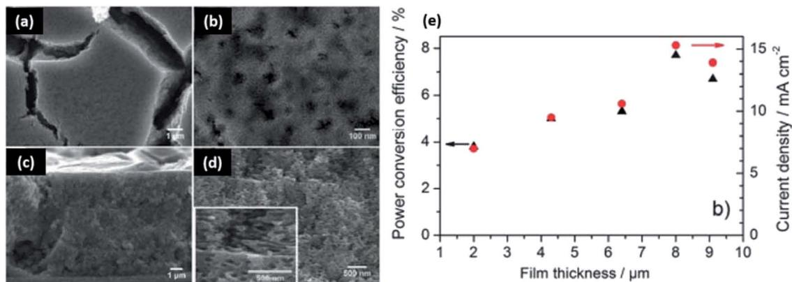
Fig. 7 Porous structures of titanium dioxide in ethyl cellulose matrices with Pluronic 127 surfactant for power conversion. SEM micrographs of (a) film morphology prior to calcination, (b) film morphology after calcination, (c) cross-section before calcination, (d) cross-section after calcination, and (e) the optoelectronic properties as a function of film thickness. This figure was adapted from ref. 151 with permission from Elsevier, 2014.
