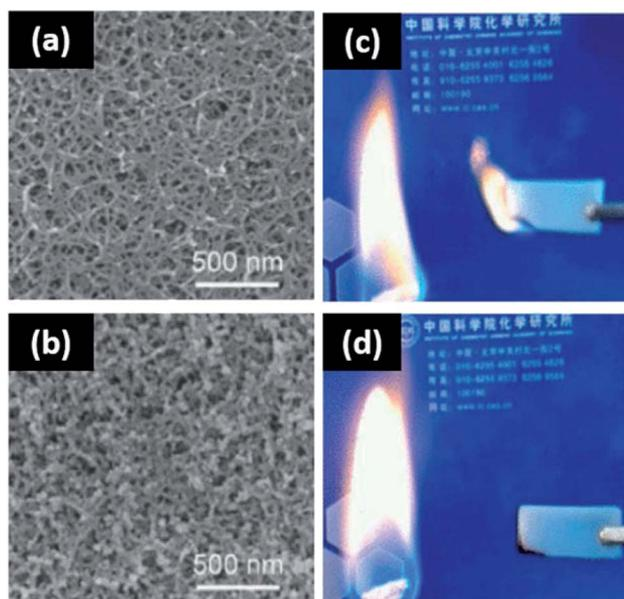
Fig. 3 Templated assembly of silica nanoparticles *via* CO<sub>2</sub> drying for flame retardancy. (a) SEM micrograph of cellulose-only aerogel; (b) SEM micrograph of cellulose-silica composite aerogel; (c) flame repellency of the cellulose-only aerogel; (d) cellulose-templated silica aerogel. This figure has been adapted from ref. 221 with permission from the American Chemical Society, 2017.
