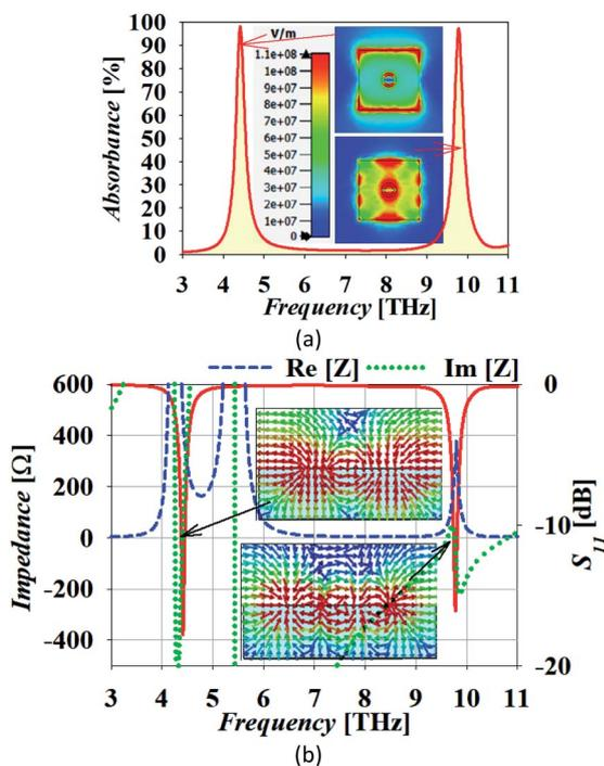
Fig. 2 (a) The absorption spectrum and contour plot of the absolute electric field in the  $xy$ -plane and (b) the impedance plot and vectored electric field ( $E_x$ -magnitude) in the  $xz$ -plane of unit-cell at  $y = 0$   $\mu\text{m}$ .
