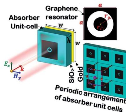
Fig. 1 The absorber unit cell, graphene resonator and its periodic arrangement ( $a = 5$ ,  $r_o = 0.6$ ,  $r_i = 0.4$ ,  $w = 9$ ,  $h = 2.5 \mu\text{m}$ ,  $\mu_c = 0.4 \text{ eV}$ ,  $T = 300 \text{ K}$ ,  $\tau = 0.1 \text{ ps}$  and graphene thickness,  $t_g = 0.34 \text{ nm}$ ).
