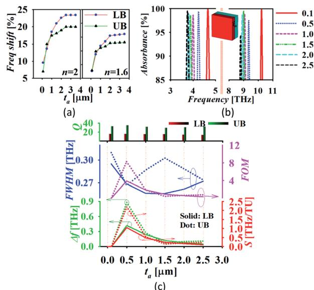
Fig. 7 (a) The frequency shift, (b) the absorption spectrum with the variation in  $t_a$  and (c) absorption performance analysis (LB: lower band and UB: upper band).
