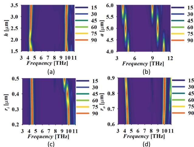
Fig. 5 The absorber response with the variation in (a)  $h$ , (b)  $a$ , (c)  $r_i$  and (d)  $r_o$  (all the dimensions are in  $\mu\text{m}$ ).
