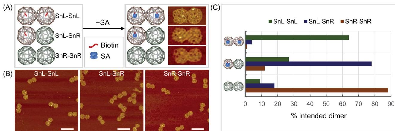
**Fig. 3** Validation of chirality. (A) Schematic diagrams (left) and AFM results after reaction with biotin (right) showing the different produced Sn dimers, biotin modifications and SA attachment where SA is visible in AFM images as white dots. (B) Wider field AFM images of the 3 forms of Sn dimers after reaction with biotin for bound SA with dimer structures of SnL–SnL (left), SnL–SnR (middle) and SnR–SnR (right). (C) Quantitation of intended dimers formed. AFM scale bars represent 200 nm.
