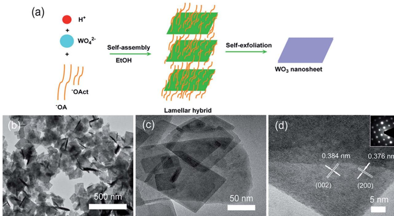
Fig. 3 (a) Schematic of self-assembly. (b–d) SEM, TEM, and HRTEM images of  $\text{WO}_3$  nanosheets produced with a NaOct/NaOA mass ratio of 0.04. Reprinted with permission from ref. 53, copyright 2018, Elsevier.
