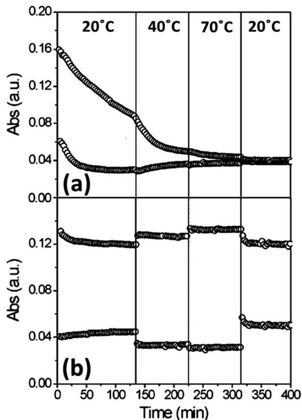
Fig. 13 Absorption change of amorphous (a) and crystalline (b)  $\text{WO}_3$  thin films at various temperatures over time. Reprinted with permission from ref. 96, copyright 2007, American Chemical Society.
