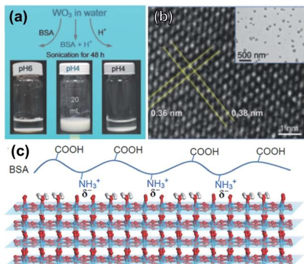
Fig. 7 (a) Optimization of exfoliation/purification for  $\text{WO}_3$  exfoliation. (b) HRTEM of a nanosheet with lattice spacing indicated; inset shows typical lateral size of  $\text{WO}_3$  nanosheets. (c) Schematic illustration for electrostatic-driven interaction of BSA on  $\text{WO}_3$  surface. Reprinted with permission from ref. 16, copyright 2017 John Wiley and Sons.
