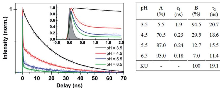
Fig. 3 (Left panel) Time-resolved fluorescence data for Au<sub>102</sub>-KU hybrid at different pH values. Thick solid lines are deconvolution fits with two exponential functions (see ES11†) to the experimental data points. Inset shows expanded view of the early time dynamics for the different pH values. (Right panel) Fitted parameters from different pH decay curves in comparison with KU dye.
