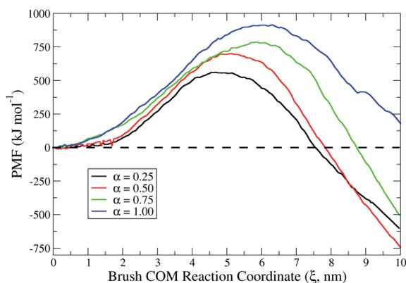
Fig. 8 Potential of mean force as a function of the reaction coordinate for lipid-adhesive brushes with varying degrees of protonation (*i.e.*  $\alpha$  ranging from 0.25 to 1) approaching and interacting with a lipid bilayer.
