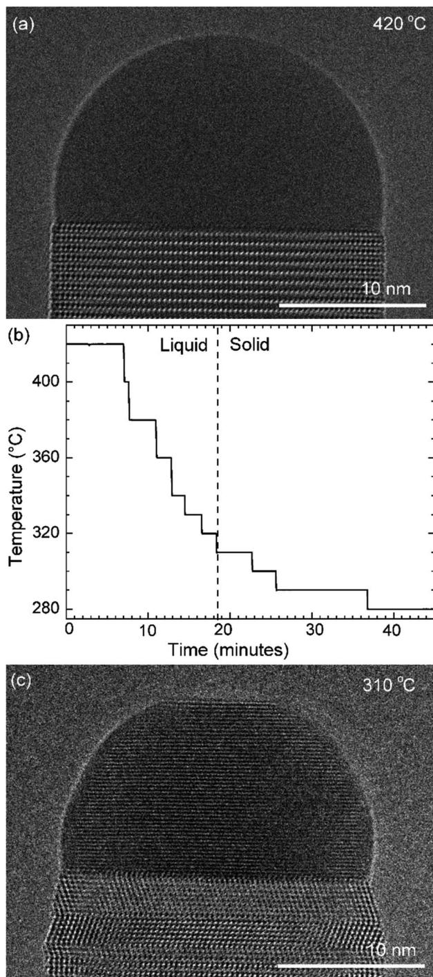
**Fig. 1** Stepwise cooling: (a) HR-TEM image of the nanowire–catalyst system during layer growth at 420 °C. At this temperature the catalyst is liquid. (b) The growth temperature was decreased in steps in this experiment. The catalyst solidified at 310 °C with one set of the crystal planes aligned parallel to the nanowire–catalyst interface. (c) TEM image where the catalyst has solidified.
