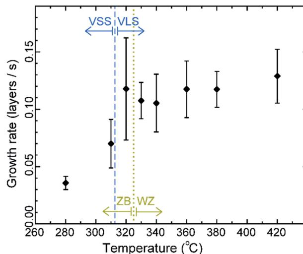
Fig. 5 Average growth rate: average growth rate of the same nanowire at different temperatures. At 310 °C and lower the catalyst is solid. The wire was growing in the wurtzite (WZ) structure at temperatures between 420 °C and 330 °C and as zinc blende (ZB) at lower temperatures. Error bars represent standard deviation.
