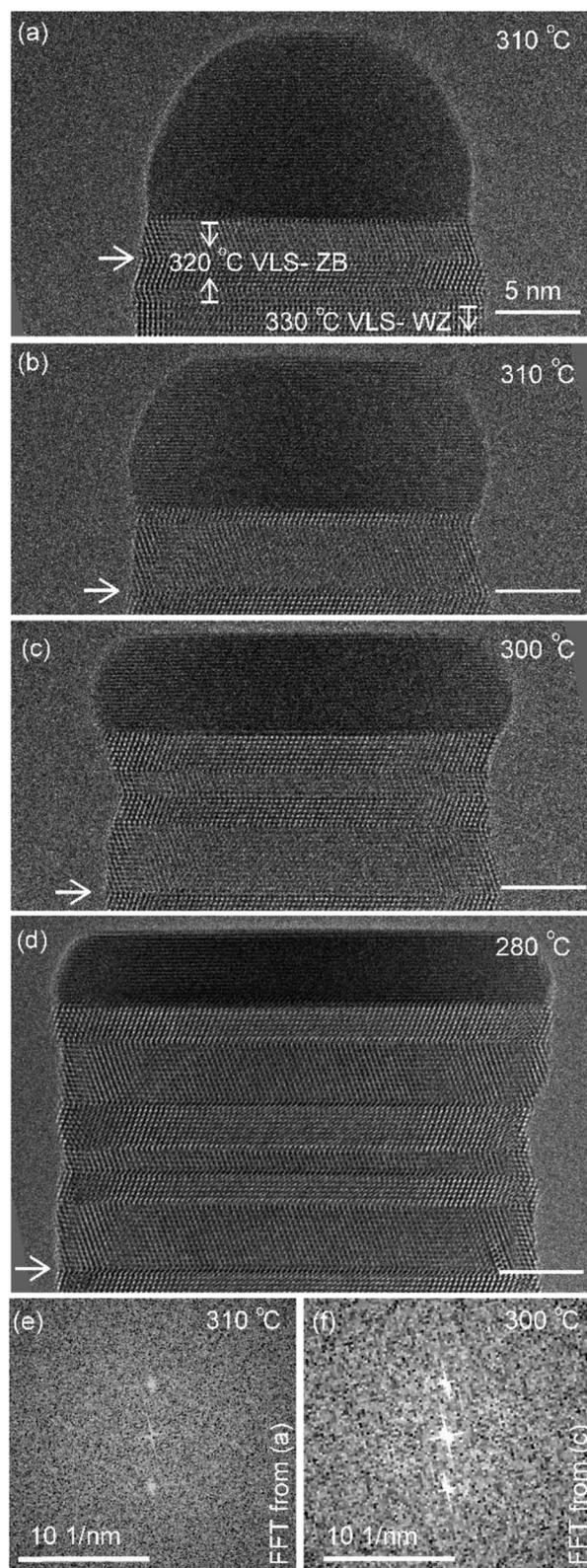
**Fig. 3** (a–d) TEM images (after averaging and rotating) of the nanowire at the same magnification at different temperatures. The arrow marks the same defects in all the images. Scale bar is 5 nm in (a–d). Power spectrum/Fast-Fourier-Transform (FFT) of the catalyst region from images (a) and (c) are given as (e) and (f) respectively.
