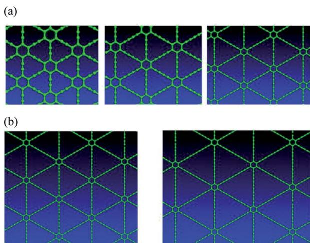
**Fig. 1** (a) Top views of  $\gamma$ -type graphyne- $n$  varieties, where  $n$  indicates the number of carbon–carbon triple bonds in a link between two adjacent hexagons. Graphyne is graphyne-1 (left), graphdiyne is graphyne-2 (middle), and graphyne-3 (right); (b) top views of  $\gamma$ -type graphyne-4 (left) and graphyne-5 (right) 2D nanostructures.
