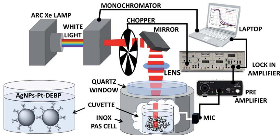
Fig. 1 Experimental setup of photoacoustic spectroscopy (PAS). The light absorbed by the AgNPs is converted into heat, generating an acoustic pressure finally detected by a microphone. In the inset, the chemical structure of the functionalized AgNP sample used in this work is shown.
