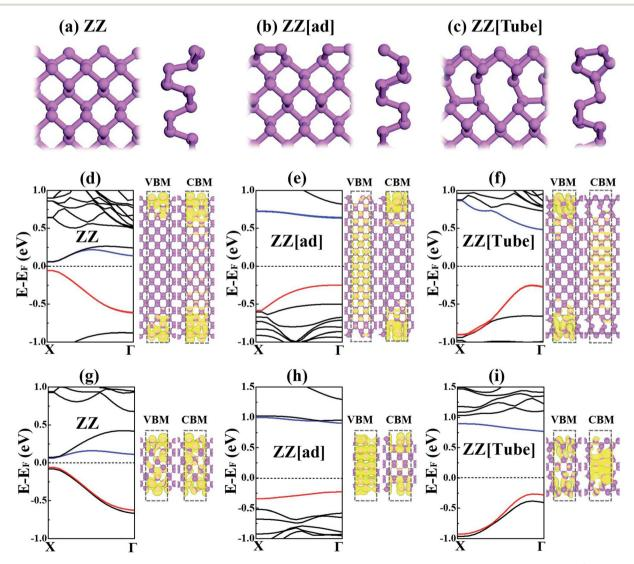
Fig. 1 The geometries of zigzag PNRs with different edge structures (a-c) and the band structures of PNRs with a width of 40 Å (d-f) and with a width of 15 Å (g-i). The highest valance band and lowest conductive band are labeled in red and blue, respectively. The charge contributions to VBM and CBM are presented beside each band structure with an isosurface value of  $1.2 \times 10^{-4}$  |e| bohr<sup>-3</sup>.
