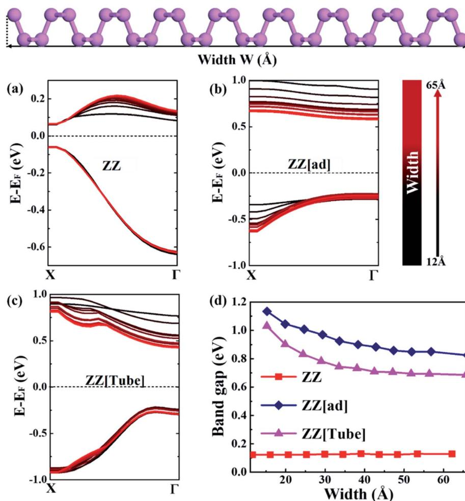
Fig. 2 The changes in VBM and CBM with ribbon width for ZZ, ZZ[ad] and ZZ[Tube] PNRs (a–c). The horizontal dashed lines indicate the Fermi level. The band gaps of ZZ, ZZ[ad] and ZZ[Tube] PNRs are a function of ribbon width (d). At the top, a schematic diagram is presented showing the definition of the ribbon width.
