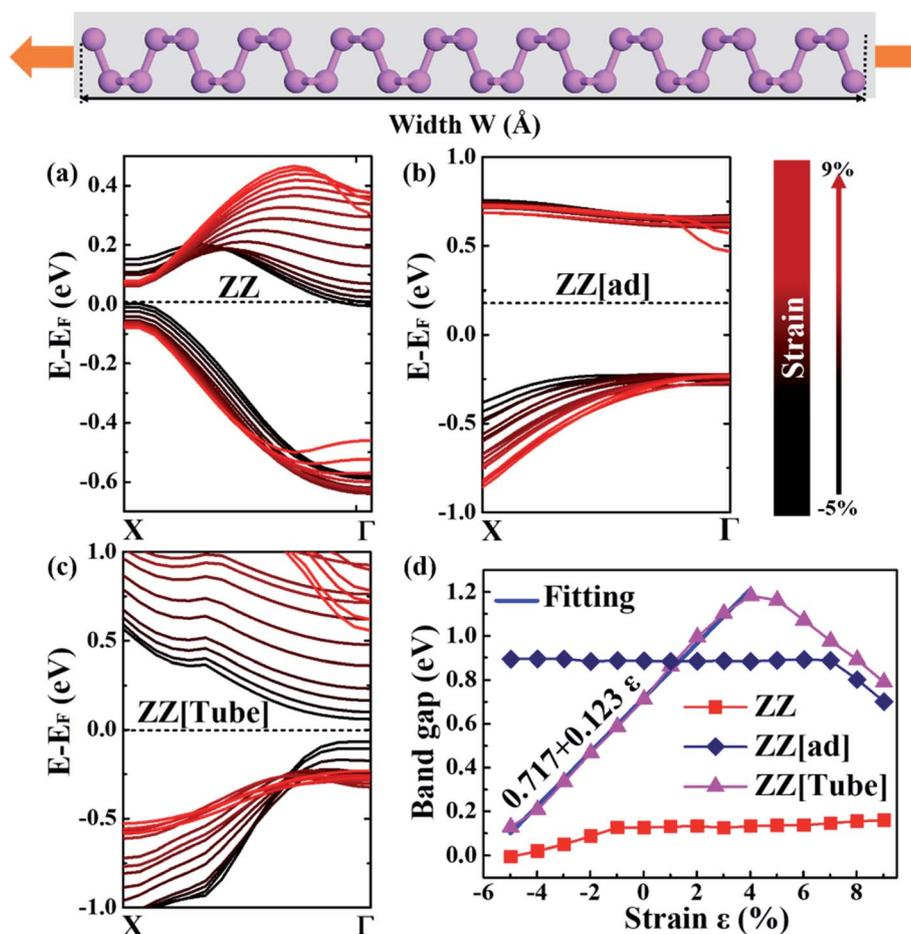
Fig. 4 The changes in VBM and CBM with strain for ZZ, ZZ[ad] and ZZ[Tube] PNRs with a width of 40 Å (a–c). The horizontal dashed lines indicate the Fermi level. The band gaps of ZZ, ZZ[ad] and ZZ[Tube] PNRs are a function of strain (d). The solid blue line is the linear fitting of the relation between the band gap  $E_g$  and the strain  $\epsilon$ .
