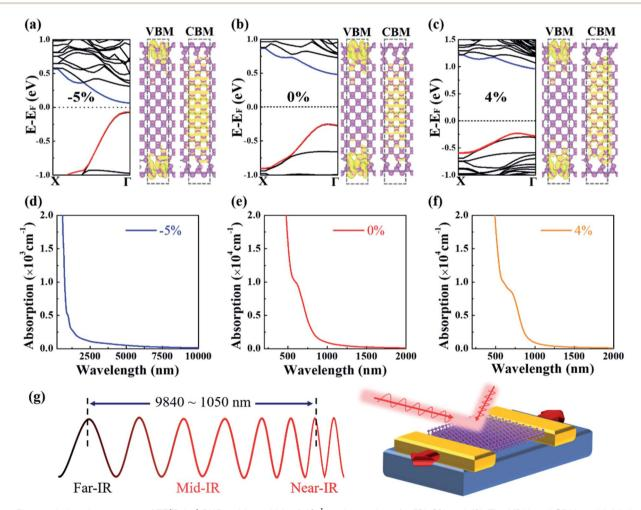
Fig. 5 Electronic band structures of ZZ[Tube] PNRs with a width of 40 Å under strains of -5%, 0% and 4%. The VBM and CBM are highlighted in red and blue, respectively. The isosurface value is  $1.2 \times 10^{-4}$  [e] bohr<sup>-3</sup> (a-c). The VBM and CBM are highlighted in red and blue, respectively. (d)– (f) Optical absorption coefficients of ZZ[Tube] PNRs under strain at -5%, 0% and 4%. (g) A schematic diagram of a possible optoelectronics application of ZZ[Tube] PNRs.
