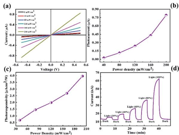
Fig. 5 CdMoS<sub>4</sub> nanoflower-based photodetector device (a) current–voltage ( $I$ – $V$ ) characteristics, (b) photocurrent as a function of power density, (c) photoresponsivity vs. power density and (d) current–time ( $I$ – $t$ ) plot.
