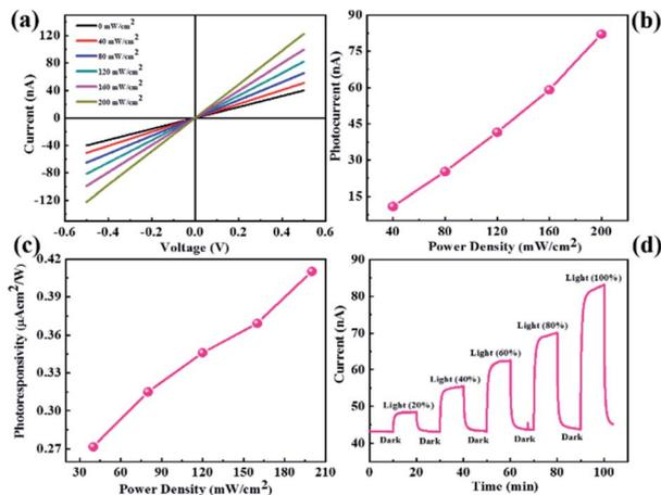
Fig. 4 MoS<sub>2</sub> nanosheet-based photodetector device. (a) current–voltage ( $I$ – $V$ ) characteristics, (b) photocurrent as a function of power density, (c) photoresponsivity vs. power density and (d) current–time ( $I$ – $t$ ) plot.
