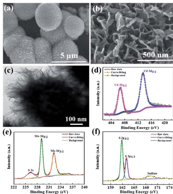
Fig. 3 (a and b) FESEM images, (c) TEM image and (d–f) deconvoluted XPS spectra for Cd 3d, Mo 3d, and S 2p of the CdMoS<sub>4</sub> nanoflowers annealed at 400 °C.
