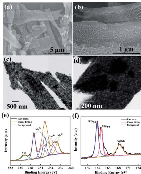
Fig. 2 (a and b) FESEM images, (c and d) TEM images and (e and f) deconvoluted XPS spectra for Mo 3d and S 2p elements of the MoS<sub>2</sub> samples annealed at 400 °C.
