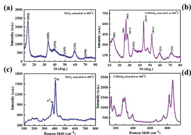
Fig. 1 XRD pattern of (a) MoS<sub>2</sub> and (b) CdMoS<sub>4</sub> samples annealed at 400 °C, Raman spectra of (c) MoS<sub>2</sub> and (d) CdMoS<sub>4</sub> samples annealed at 400 °C.
