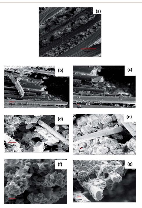
Fig. 5 Fractured SEM images of (a–c) epoxy/CF, (d and e) epoxy/CF laminates containing GO, and (f and g) epoxy/CF laminates containing HPEEK-g-GO.<sup>55</sup> Reproduced from ref. 55 with permission from Elsevier (2018).
