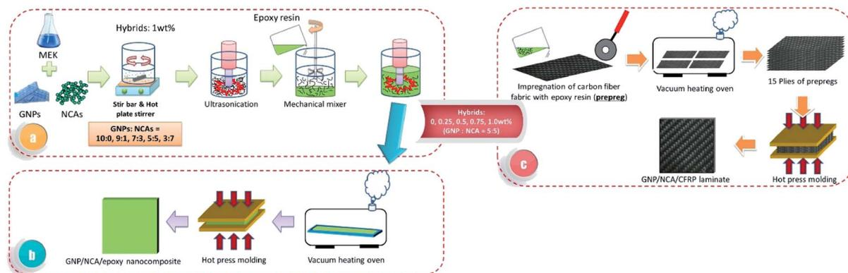
Fig. 3 Preparation of the carbon hybrid/nano-composites and CFRE laminates.<sup>48</sup> Reproduced from ref. 48 with permission from Elsevier (2019).
