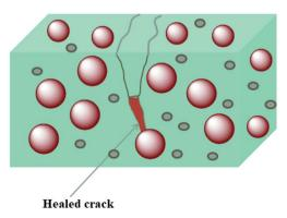
Fig. 13 Schematic depicting the concept of microcapsules and their self-healing action.
