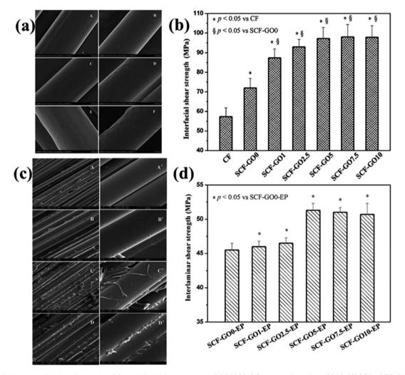
Fig. 10 (a) SEM images of carbon fibers after GO modified sizing treatment: (A) T700S; (B) virgin carbon fibers (CFs); (C) SCF-GO0; (D) SCF-GO1; (E) SCF-GO5; and (F) SCF-GO10. (b) IFSS of the resulting composites; (c) fracture surface micrographs of carbon fiber/epoxy composites: (A and A') SCF-GO0-EP; (B and B') SCF-GO1-EP; (C and C') SCF-GO5-EP; (D and D') SCF-GO10-EP; (d) ILSS of the resulting composites.93 Reproduced from ref. 93 with permission from ACS (2012).
