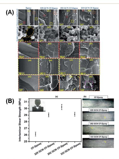
Fig. 4 (A) SEM images of the fractured surface cross-sections both along and transverse to the direction of the applied load for (a(1-5)) CFepoxy, (b(1-5)) 25Gr:25CNT:50ND CF-epoxy, (c(1-5)) 25Gr:50CNT:25ND CF-epoxy and (d(1-5)) 33Gr:33CNT:33ND CF-epoxy composites at different magnifications. (B) ILSS plots for CF-epoxy and various combinations of the Gr:CNT:ND CF-epoxy composite.54 Reproduced from ref. 54 with permission from Elsevier (2019).
