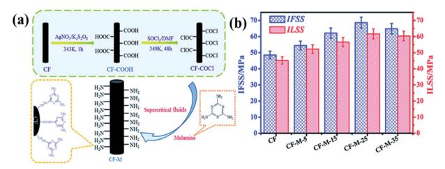
Fig. 7 (a) Schematic of the chemical functionalization of melamine over carbon fibers and (b) improvement in IFSS and ILSS properties with grafting time.<sup>82</sup> Reproduced from ref. 82 with permission from RSC (2016).
