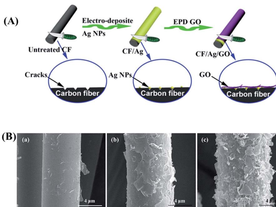
Fig. 11 (A) Schematic of surface modification of carbon fibers with Ag/GO and (B) SEM micrographs showing the increase in surface roughness with subsequent modifications.<sup>97</sup> Reproduced from ref. 97 with permission from Elsevier (2017).
