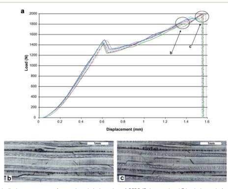
Fig. 14 (a) Typical load-displacement curves for quasi-static indentation of CFRP (3 damaged and 3 healed samples), cross-sectional damage for impact force (b) 1700 N and (c) 2000 N.<sup>116</sup> Reproduced from ref. 116 with permission from Elsevier (2007).
