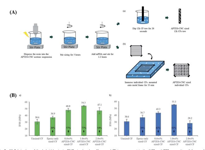
Fig. 9 (A) Fabrication of the hybrid laminate CNC-sized carbon fibers and (B) improvement in the ILSS and IFSS properties of the resulting composites.<sup>88</sup> Reproduced with permission from Elsevier (2018).
