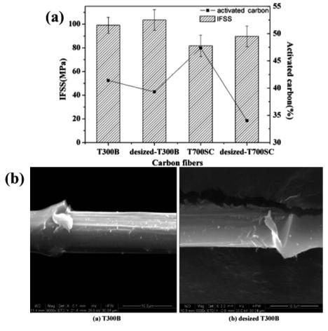
Fig. 1 (a) Bar diagram representing the change in IFSS on desizing of carbon fibers and (b) SEM micrograph showing the increased surface roughness post desizing.<sup>33</sup> Reproduced from ref. 33 with permission from Elsevier (2011).
