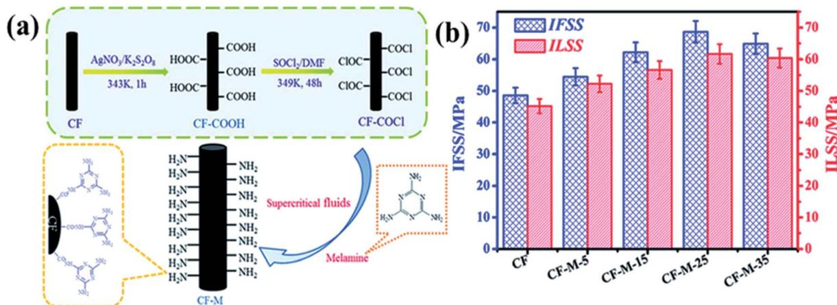
Fig. 7 (a) Schematic of the chemical functionalization of melamine over carbon fibers and (b) improvement in IFSS and ILSS properties with grafting time.<sup>82</sup> Reproduced from ref. 82 with permission from RSC (2016).
