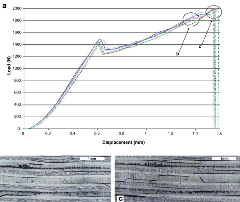
Fig. 14 (a) Typical load–displacement curves for quasi-static indentation of CFRP (3 damaged and 3 healed samples), cross-sectional damage for impact force (b) 1700 N and (c) 2000 N.<sup>116</sup> Reproduced from ref. 116 with permission from Elsevier (2007).
