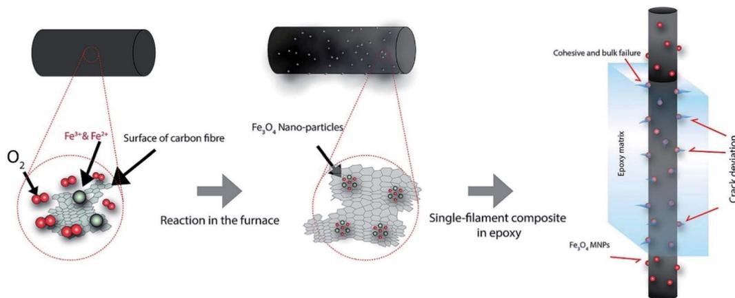
Fig. 12 Schematic of  $\text{Fe}_3\text{O}_4$  nanoparticle growth over carbon fibres and their subsequent effect of better mechanical interlocking with epoxy.<sup>101</sup> Reproduced from ref. 101 with permission from Elsevier (2019).
