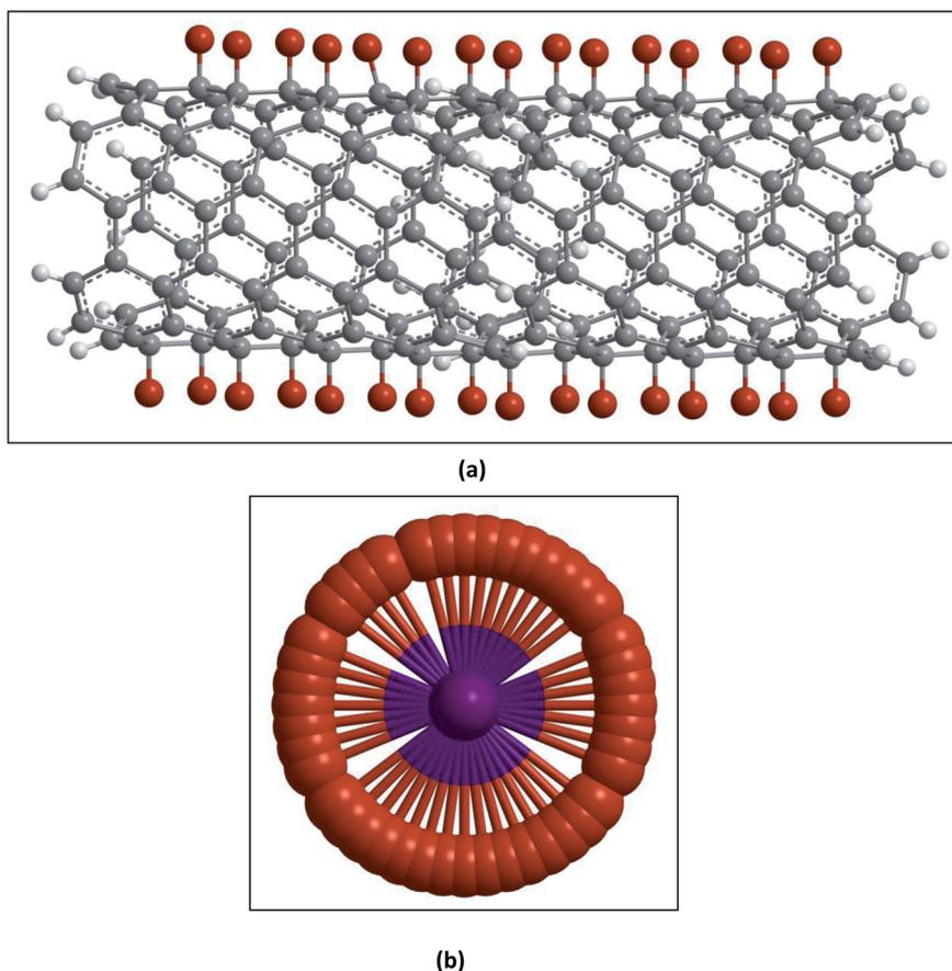
Fig. 9 Surfactant functionalization of CNTs (a) and a surfactant micelle (b).
