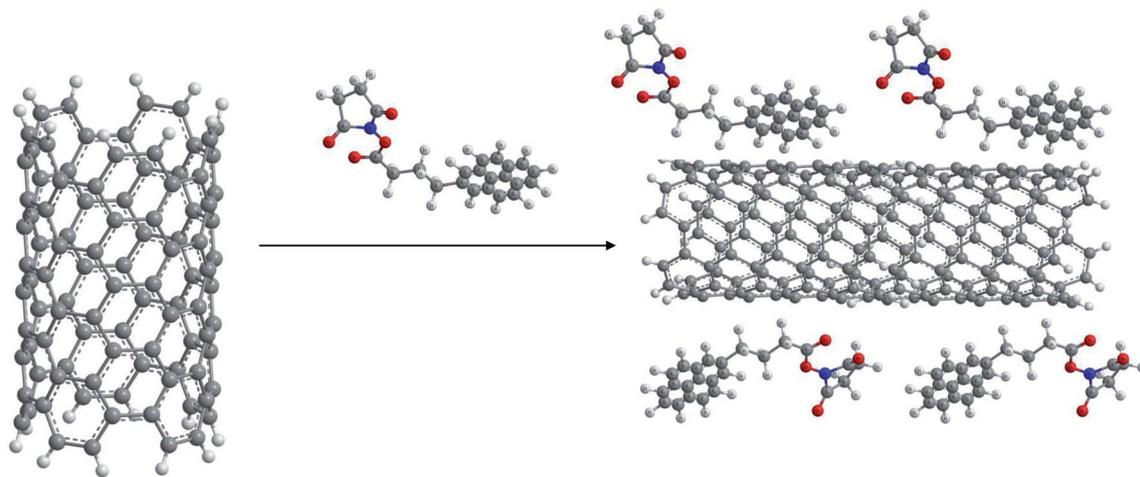
Fig. 11 Functionalization of CNTs by substituted pyrenes.
