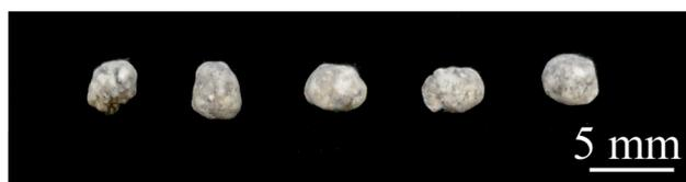
Fig. 1 Photograph of commercial diammonium phosphate (c-DAP) granules. Bar depicts 5 mm.
