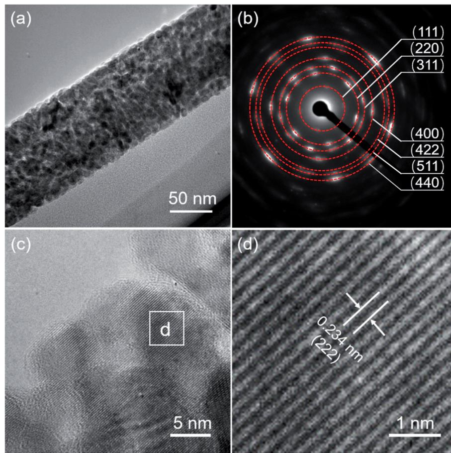
Fig. 2 TEM characterization of a  $\text{MnCo}_2\text{O}_{4.5}$  NW removed from the SSF substrate: (a) TEM image, (b) related SAED pattern, (c) high-resolution TEM image, and (d) magnified high-resolution TEM image from the selected position in (c).
