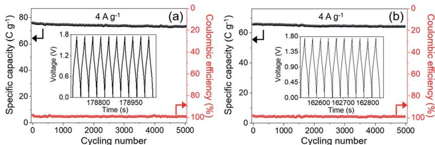
Fig. 9 Cycling tests and coulombic efficiency of (a)  $\text{MnCo}_2\text{O}_{4.5}$  NWs//AC and (b)  $\text{MnCo}_2\text{O}_{4.5}$  QCs//AC HSCs during 5000 cycles at  $4 \text{ A g}^{-1}$ , and the insets provide the last ten GCD curves.
