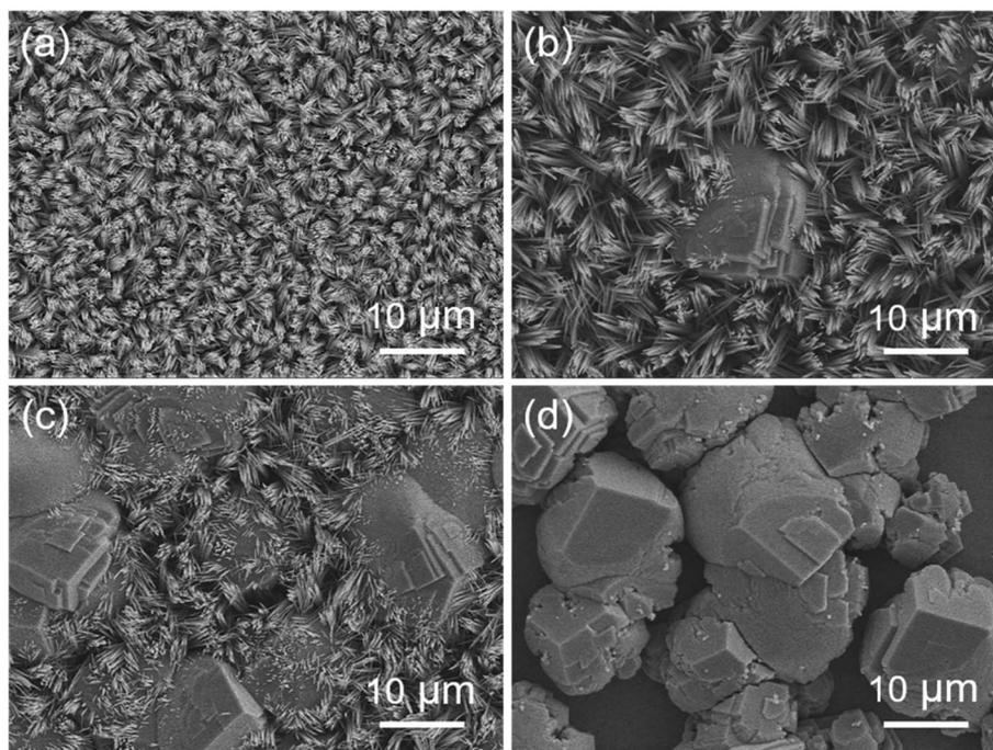
Fig. 4 SEM images of  $\text{MnCo}_2\text{O}_{4.5}$  samples prepared at different hydrothermal temperatures of (a) 100, (b) 130, (c) 140, and (d) 150 °C, respectively. All samples were processed with an annealing treatment at 400 °C for 3 h.
