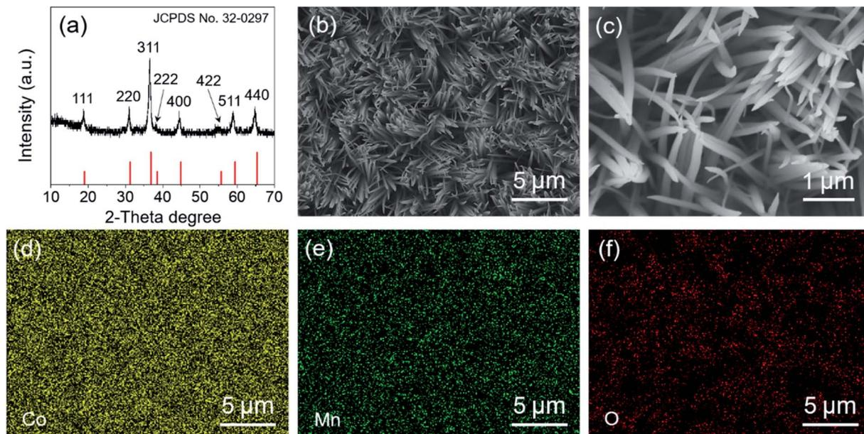
Fig. 1 Crystal phase and morphological investigations of the SSF-supported  $\text{MnCo}_2\text{O}_{4.5}$  NWs prepared at  $120^\circ\text{C}$  for 6 h followed by an annealing treatment at  $400^\circ\text{C}$  for 3 h: (a) XRD pattern, (b and c) SEM images at different magnifications, and the related EDS elemental mapping images taken from the position of (b) for (d) Co, (e) Mn, and (f) O, respectively.
