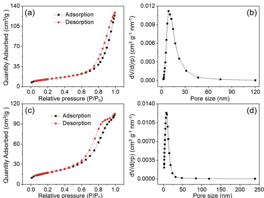
Fig. 5 (a) Nitrogen adsorption–desorption isotherms and (b) the related BJH pore size of MnCo<sub>2</sub>O<sub>4.5</sub> NWs obtained at 120 °C, and (c) nitrogen adsorption–desorption isotherms and (d) the related BJH pore size of MnCo<sub>2</sub>O<sub>4.5</sub> QCs obtained at 150 °C.
