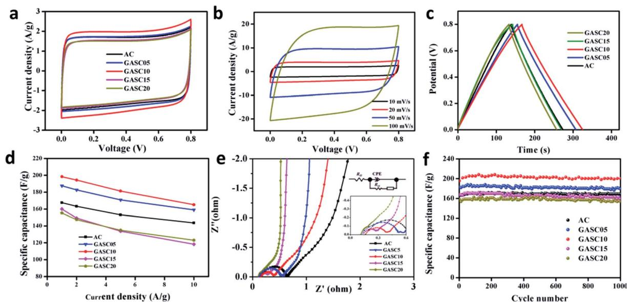
Fig. 5 Electrochemical performance of SCs based on AC, GASC05, GASC10, GASC15, and GASC20 samples in 6 M KOH solution. (a) CV curves at a scan rate of 10 mV s<sup>-1</sup>; (b) CV curves of GASC10 at different scan rates between 10 mV s<sup>-1</sup> and 100 mV s<sup>-1</sup>; (c) charge–discharge curves at a current density of 1 A g<sup>-1</sup>; (d) specific capacitances at various current densities; (e) Nyquist plots; (f) cycling performance at 1 A g<sup>-1</sup>.
