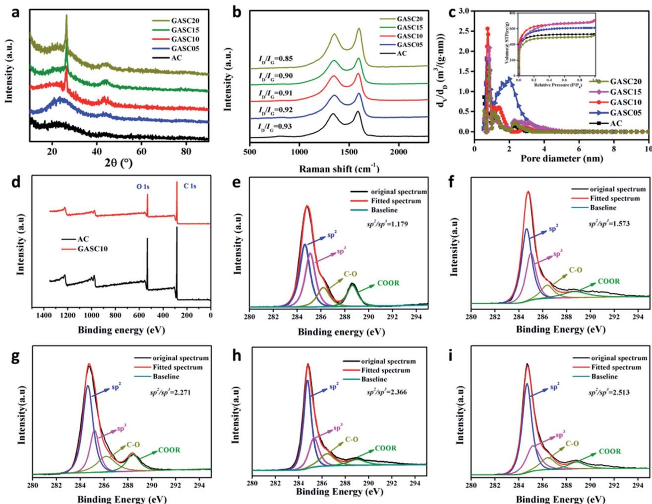
Fig. 3 (a) XRD patterns, (b) Raman spectra, (c) pore size distributions and  $N_2$  adsorption–desorption isotherms (inset) of GASC samples; (d) XPS survey spectra of AC and GASC10; (e–i) high resolution C 1s spectra of AC (e), GASC05 (f), GASC10 (g), GASC15 (h), and GASC20 (i).
