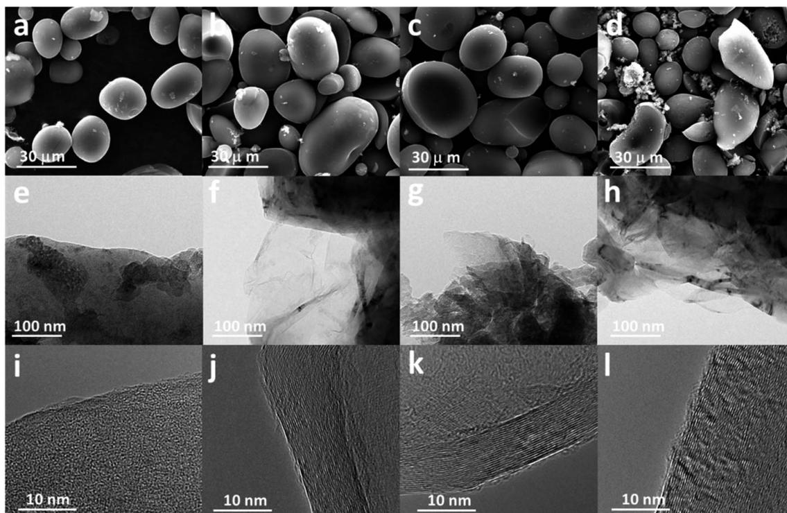
Fig. 2 SEM, TEM, and HRTEM images of AC (a, e and i), GASC5 (b, f and j), GASC10 (c, g and k), and GASC15 (d, h and l).
