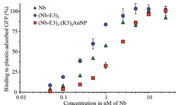
Fig. 5 Apparent binding abilities of the GFP-binding nanobody (green triangle), and the dimerized  $(Nb-E3)_2$  (blue dot) and the non-covalent  $(Nb-E3)_2:(K3)_2$ AuNP assemblies (red square). The binding to GFP was determined using indirect ELISA analysis and plate-adsorbed GFP
