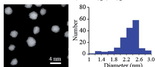
Fig. 4 Characterization of the non-covalent  $(Nb-E3)_2:(K3)_2$ AuNP assemblies. (A) Native PAGE analysis results to determine the average stoichiometry for the complete assembly of  $(Nb-E3)_2$  with  $(K3)_2$ AuNPs. (B) Scanning transmission electron microscopy (STEM) analysis results of the  $(Nb-E3)_2:(K3)_2$ AuNP.
