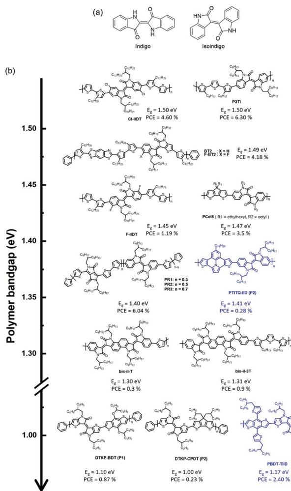
Fig. 7 (a) Chemical structure of indigo, isoindigo and (b) isoindigo-based polymers.
