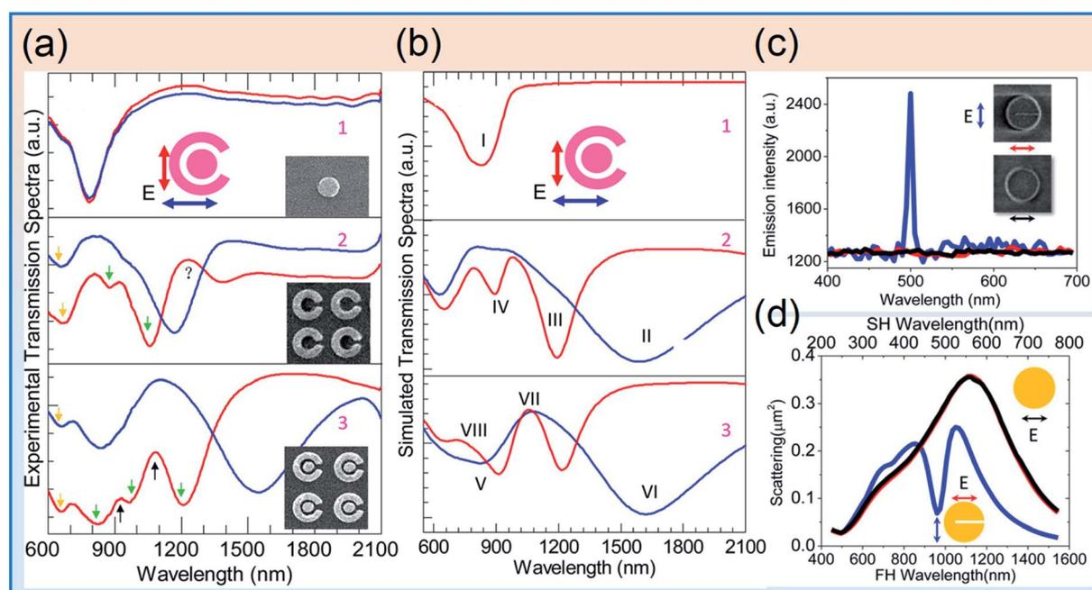
Fig. 8 (a and b) Experimental (a) and calculated (b) transmission spectra of disk (1), SRR (2), and SRR/D (3) arrays.<sup>116</sup> (c and d) Measured SH emission and SH emission intensity versus the incident wavelength (c) and calculated scattering spectra (d) for the single split and perfect nanodisks<sup>119</sup> (reproduced with permission from ref. 116 Copyright 2013 and ref. 119 Copyright 2016, the American Chemical Society).
