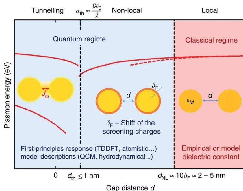
Fig. 7 The impact of quantum mechanical effects on plasmonic resonances<sup>113</sup> (reproduced with permission from Copyright 2016, the Authors).
