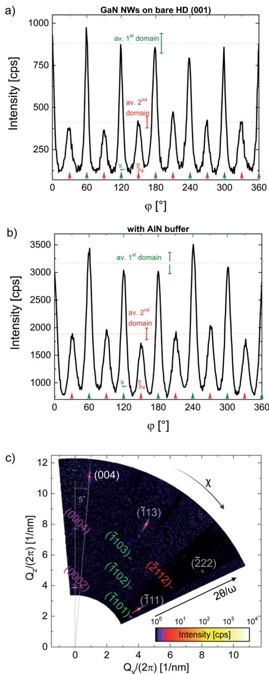
**Fig. 5** XRD of GaN NWs on HD (001):  $\phi$ -scan of the asymmetric (1103) reflex of GaN NWs on (a) bare diamond and (b) with the AlN buffer layer. (c) RSM of GaN NWs grown on AlN-buffered HD (001). The symmetric GaN (diamond) reflexes are labeled in violet (white), while the asymmetric ones are labeled in green and red (gray). The dashed gray lines indicate the angle between [0001]GaN and [001]diamond.
