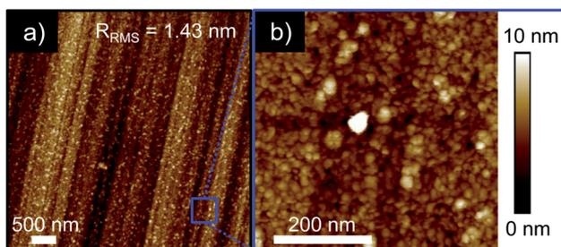
Fig. 1 (a) 5 × 5 μm<sup>2</sup> and (b) 500 × 500 nm<sup>2</sup> AFM images of the AlN buffer layer on HD (001).
