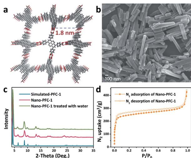
Fig. 1 (a) The two-dimensional porous structure of PFC-1. (b) A scanning electron microscopy (SEM) image, (c) powder XRD patterns, and (d) the  $N_2$  adsorption/desorption isotherm (77 K) of Nano-PFC-1.
