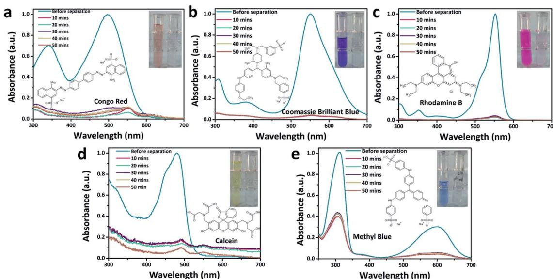
Fig. 4 The chemical structures of the dyes, digital photos, and UV-vis spectra of the feed (blue lines) and permeate (lines in other colors) solutions: (a) Congo red, (b) Coomassie brilliant blue, (c) rhodamine B, (d) calcein, and (e) methyl blue.
