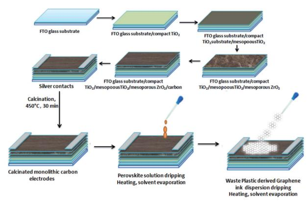
Fig. 7 Schematic of the device fabrication of the HTM free PSC with 3D GNs.
