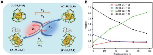
Fig. 14 Amplification of the enantiomeric excess after introducing chiral R-BINAS to the Au<sub>38</sub> nanoclusters. (A) Scheme for the dynamic inversion system, (B) evolution of different clusters species under 70 °C as a function of time. The nomenclature of the four different species assigned as follow: (A-38, 24, R-0) corresponded to A-Au<sub>38</sub>(2-PET)<sub>24</sub>; Adapted with permission from ref. 16. Copyright 2020 Nature Research.
