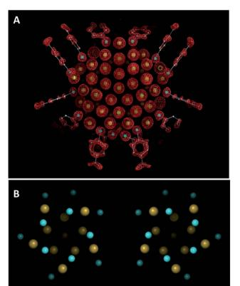
Fig. 2 X-ray crystal structure of the Au<sub>102</sub>(p-MBA)<sub>44</sub> crystal. (A) Electron density map and atomic structure (Au atoms depicted as yellow spheres, and p-MBA shown as framework and with small spheres [S in cyan, C in gray, and O in red]). (B) Top view of the two enantiomeric clusters. Colour scheme as in (A), only the sulfur atoms of p-MBA are shown. Adapted with permission from ref. 48. Copyright 2007 American Association for the Advancement of Science.
