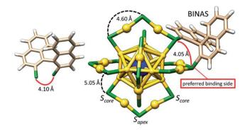
Fig. 11 3D sketch of S-BINAS (left) and MAu<sub>24</sub>(SR)<sub>16</sub>(S-BINAS)<sub>1</sub> (right), where M = Pt, Pd. Other ligands apart from BINAS are omitted for clarity. The two types of sulfur environments are indicated with Score (also called terminal) and  $S_{apex}$  (also called central). Color code: Au =yellow, S = green, C = beige, H = white, Pt and Pd = blue. Adapted with permission from ref. 103. Copyright 2017 American Chemical Society
