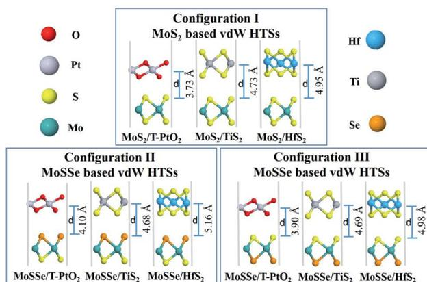
Fig. 2 vdW HTSs with configurations I, II and III. MoS<sub>2</sub>/BX<sub>2</sub> (configuration I), MoSSe/BX<sub>2</sub> (configuration II), where the Se atomic layer is at the interface, and MoSSe/BX<sub>2</sub> (configuration III), where the S atomic layer is at the interface.
