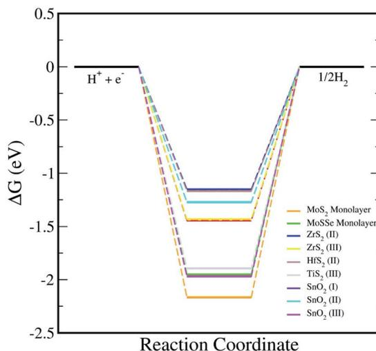
Fig. 6 The HER reaction free energy diagrams on the monolayers and vdW HTSs at an electrode potential  $E_{\text{SHE}} = 0$  V and pH = 0. At zero potential, ( $\text{H}^+ + \text{e}^-$ ) can be expressed as  $1/2\text{H}_2$ .
