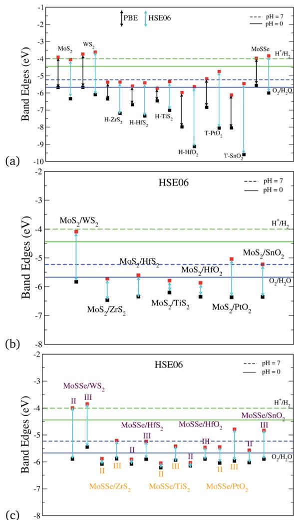
Fig. 3 Band edge alignment with respect to water redox potentials of (a) the individual monolayers, (b)  $\text{MoS}_2/\text{BX}_2$  vdW HTSs (configuration I), (c)  $\text{MoSSe}/\text{BX}_2$  vdW HTSs (configuration II and III), where  $\text{BX}_2$  refers to  $\text{WS}_2$ ,  $\text{ZrS}_2$ ,  $\text{HfS}_2$ ,  $\text{TiS}_2$ ,  $\text{HfO}_2$ ,  $\text{PtO}_2$  or  $\text{SnO}_2$ .
