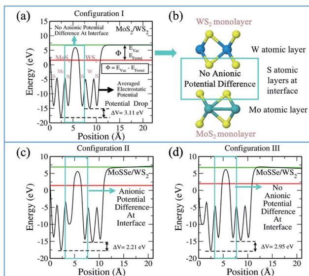
Fig. 4 Electrostatic potential plot of  $\text{MoS}_2/\text{WS}_2$  depicting (a) potential difference in configuration I, (b) schematic of configuration I; (c) potential difference in configuration II and (d) potential difference in configuration III.
