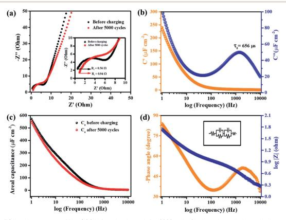
Fig. 7 (a) The EIS impedance spectra of M-nr/rGO before charging and after 2000 cycles (the inset shows the internal resistance), (b) the real component C' and the imaginary component C'' plot vs. frequency of M-nr/rGO, (c) the calculated specific capacitance of the M-nr/rGO nanocomposite from the impedance spectra before and after charging and (d) the phase angle Bode plot and impedance Bode plot of the M-nr/rGO nanocomposite.
