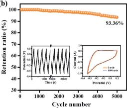
Fig. 9 (a) The Ragone plot for MnFe<sub>2</sub>O<sub>4</sub>/rGO nanoneedles (background adapted from ref. 46) and (b) cycling stability of MnFe<sub>2</sub>O<sub>4</sub>/rGO nanoneedles for 5000 cycles (inset shows the galvanostatic charge–discharge curves for a different number of cycles and CV taken at 1.5 A g<sup>-1</sup> and 5 mV s<sup>-1</sup> respectively after completing the 5000 cycles).
