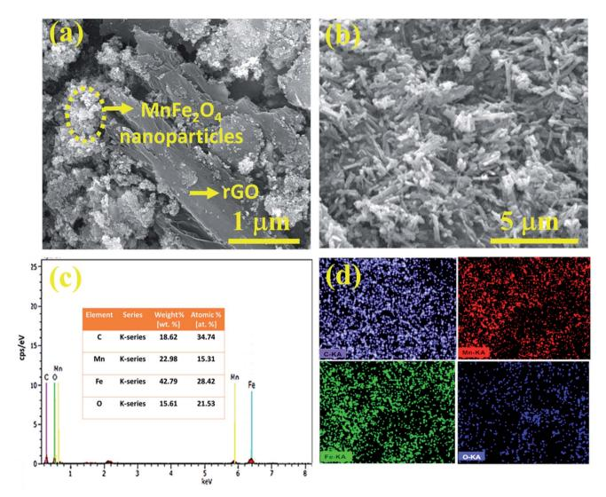
Fig. 4 FESEM image of the (a) rGO nanocomposite of MnFe<sub>2</sub>O<sub>4</sub> nanoparticles: M-np/rGO and (b) nanocomposite of MnFe<sub>2</sub>O<sub>4</sub> nanoneedles: M-np/rGO and (b) nanocomposite of MnFe<sub>2</sub>O<sub>4</sub> nanocomposite o nr/rGO, (c) EDX spectra of the MnFe<sub>2</sub>O<sub>4</sub> nanoneedle composite: M-nr/rGO (inset shows the elemental analysis based on the weight% of C, Mn, Fe and O present) and (d) the corresponding EDS mapping of the M-nr/rGO composite.
