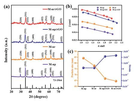
Fig. 1 (a) XRD diffraction pattern of the hydrothermally synthesized MnFe $_2$ O $_4$  nanoparticles: M-np, MnFe $_2$ O $_4$  nanoneedles: M-nr, reduced graphene oxide composite of MnFe $_2$ O $_4$  nanoparticles: M-nr/rGO, (b) Williamson–Hall (W–H) plot of the synthesized samples and (c) the relationship between particle size and strain derived from the Williamson–Hall method.
