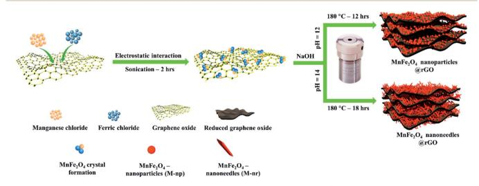
Scheme 1 Schematic illustration of hydrothermal synthesis of morphologically tuned MnFe<sub>2</sub>O<sub>4</sub>/rGO nanocomposites of nanoparticles and nanoneedles
