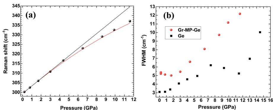
Fig. 4 (a) Peak position and (b) full width at half maximum (FWHM) of the  $T_{2g}$  mode in Gr-MP-Ge as a function of pressure (circles). The FWHM of the same mode measured on a Ge wafer is shown for comparison (square).<sup>30</sup> In (a) the black line is a linear fit of the data up to 4.5 GPa (limit of hydrostaticity) and the red curve is a quadratic fit of the dataset.
