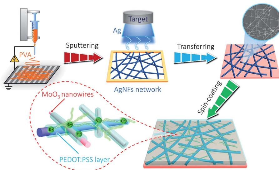
Scheme 1 The fabrication schematic of AMP film electrodes.
