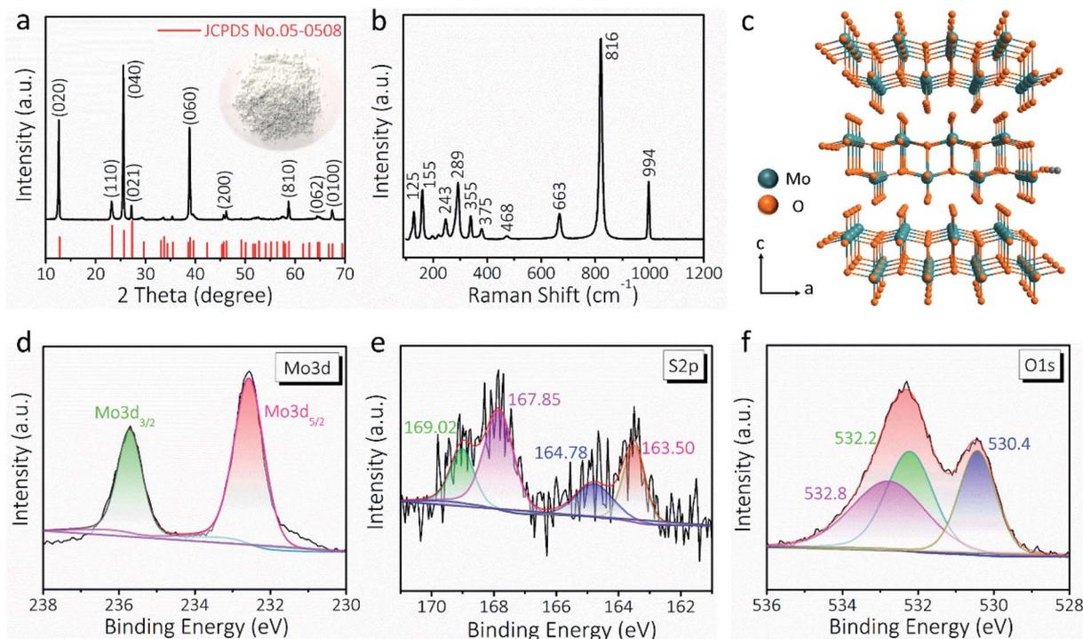
Fig. 2 (a) XRD pattern and (b) Raman spectrum of the as-synthesized MoO<sub>3</sub> nanowires (inset: a digital image of as-synthesized MoO<sub>3</sub> nanowire powder). (c) Schematic diagram of the  $\alpha$ -MoO<sub>3</sub> crystal structure. XPS spectra of (d) Mo 3d, (e) S 2p, and (f) O 1s for PEDOT:PSS-glued MoO<sub>3</sub> nanowires.
