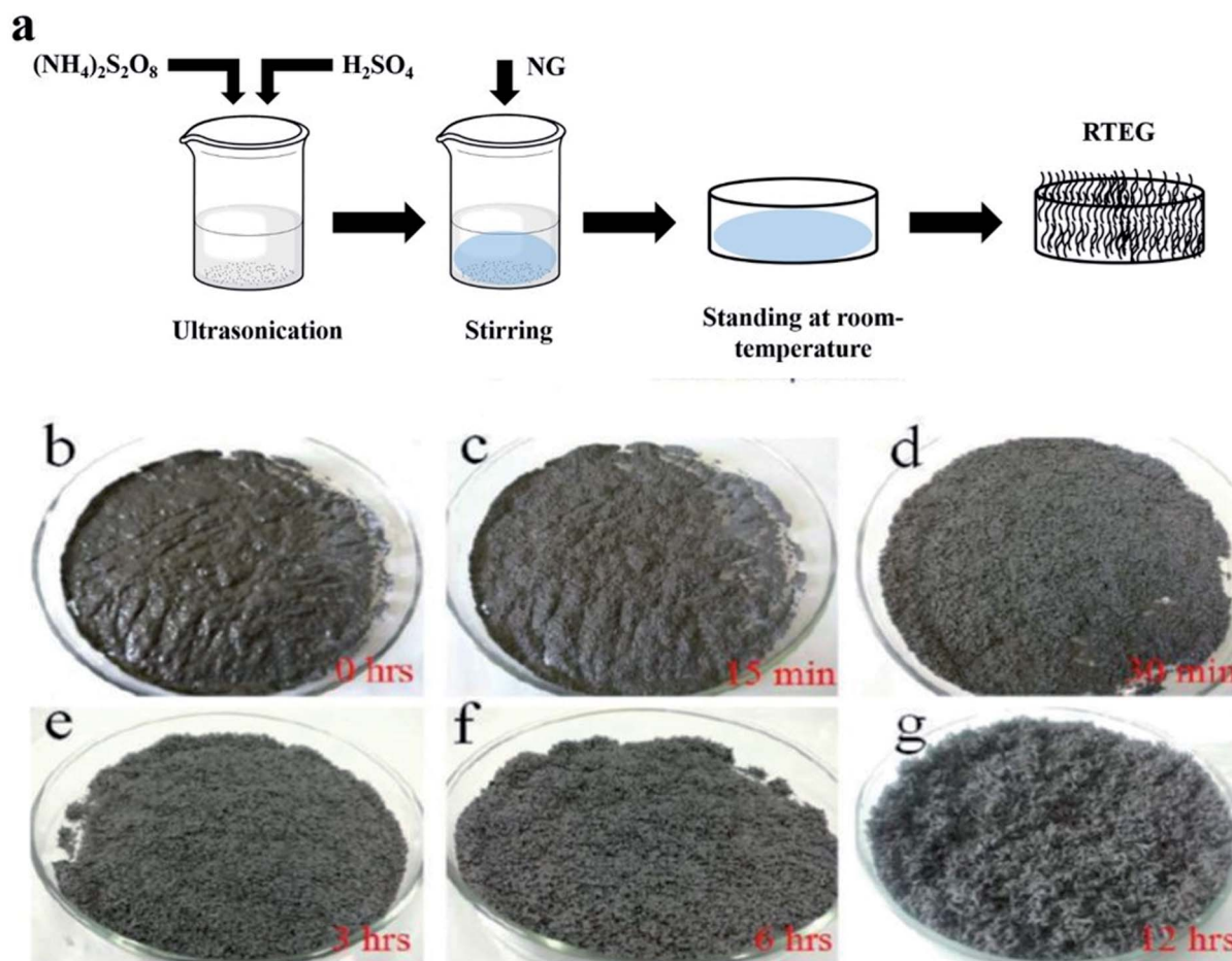
Fig. 5 (a) The schematic diagram of TEG preparation by the one-step room-temperature method. (b–g) Photographic images of the graphite intercalation and morphological evolutions with time from 0 to 12 h. 94 Adapted with permission from ref. 94 copyright 2017 Elsevier.
