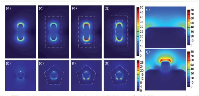
Fig. 5 FDTD simulated electric field enhancement distribution for (a and b) AuNBPs, (c and d) AuNBP@TiO2 core-shell structure, (e and f) AuNBP@TiO<sub>2</sub> nanoboxes, and (g and h) AuNBP-Pt@TiO<sub>2</sub> nanoboxes. (a), (c), (e) and (g) show the longitudinal section electric field enhancement distribution and (b), (d), (f), and (h) show the transverse one. (i and j) Partial views of the end of AuNBPs, respectively, in AuNBP@TiO2 nanoboxes and AuNBP-Pt@TiO2 nanoboxes
