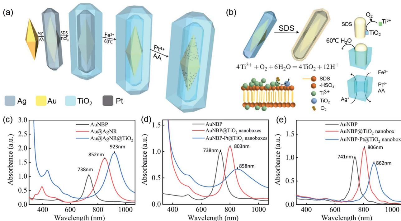
**Fig. 1** (a) The diagram of the synthesis process of the AuNBP–Pt@TiO<sub>2</sub> nanoboxes, (b) the function of the SDS soft template in the formation of the mesoporous structure, (c and d) optical absorption spectra of samples in the synthesis process, (e) FDTD-simulation optical spectra of AuNBPs, AuNBP@TiO<sub>2</sub> nanoboxes and AuNBP–Pt@TiO<sub>2</sub> nanoboxes.
