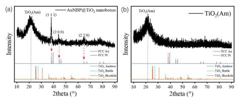
Fig. 3 XRD patterns of the (a) AuNBP@TiO<sub>2</sub> nanoboxes and (b) amorphous TiO<sub>2</sub>.
