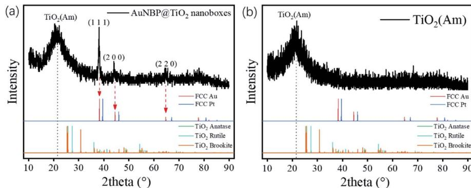
Fig. 3 XRD patterns of the (a) AuNBP@TiO<sub>2</sub> nanoboxes and (b) amorphous TiO<sub>2</sub>.
