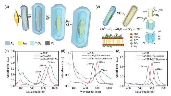
Fig. 1 (a) The diagram of the synthesis process of the AuNBP-Pt@TiO<sub>2</sub> nanoboxes, (b) the function of the SDS soft template in the formation of the mesoporous structure, (c and d) optical absorption spectra of samples in the synthesis process, (e) FDTD-simulation optical spectra of AuNBPs, AuNBP@TiO2 nanoboxes and AuNBP-Pt@TiO2 nanoboxes.
