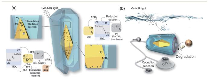
Fig. 6 (a) Photocatalysis schematic diagram and energy band diagram; (b) model analogy diagram of the platinum modified nanoboxes.
