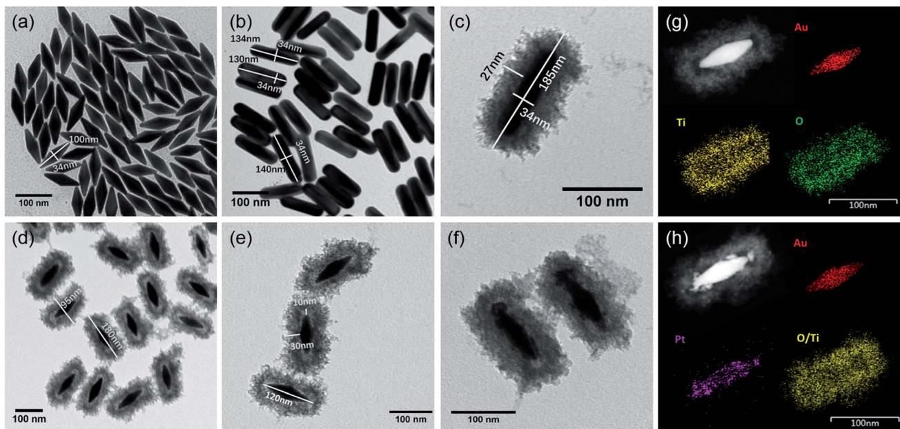
**Fig. 2** The TEM images of (a) AuNBPs, (b) Au@AgNRs, (c) Au@AgNR@TiO<sub>2</sub>, (d and e) AuNBP@TiO<sub>2</sub> nanoboxes, and (f) AuNBP–Pt@TiO<sub>2</sub> nanoboxes. (g and h) HAADF-STEM image and elemental maps of AuNBP@TiO<sub>2</sub> nanoboxes and AuNBP–Pt@TiO<sub>2</sub> nanoboxes.
