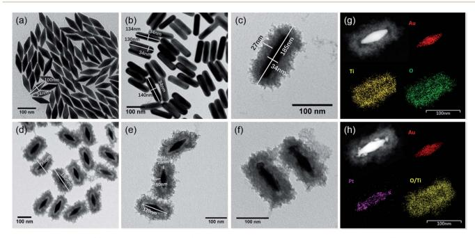
Fig. 2 The TEM images of (a) AuNBPs, (b) Au@AgNRs, (c) Au@AgNR@TiO2, (d and e) AuNBP@TiO2 nanoboxes, and (f) AuNBP-Pt@TiO2 nanoboxes. (q and h) HAADF-STEM image and elemental maps of AuNBP@TiO2 nanoboxes and AuNBP-Pt@TiO2 nanoboxes.
