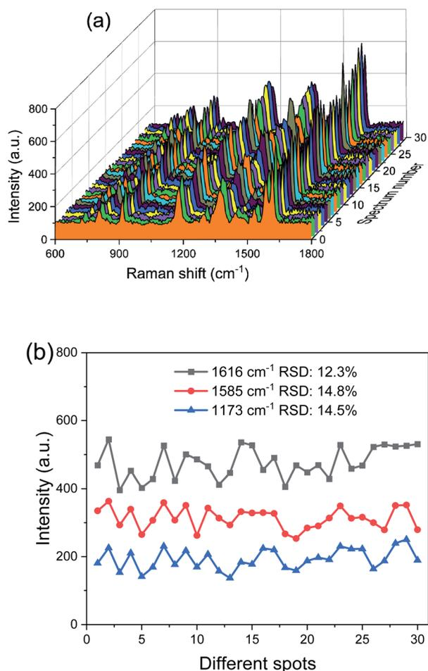
Fig. 4 (a) Raman spectra of  $10^{-5} \text{ M}$  CV at 30 different points obtained from five SERS-active capillaries. (b) the peak intensities of Raman bands at  $1173$ ,  $1585$  and  $1616 \text{ cm}^{-1}$  and the corresponding RSD values.
