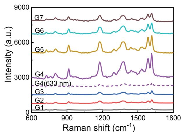
Fig. 2 Raman spectra of CV (10<sup>-5</sup> M) with different sizes of AuNPs as SERS enhancing solution. Solid lines: excited by 532 nm laser light; purple dotted line: excited by 633 nm laser light.
