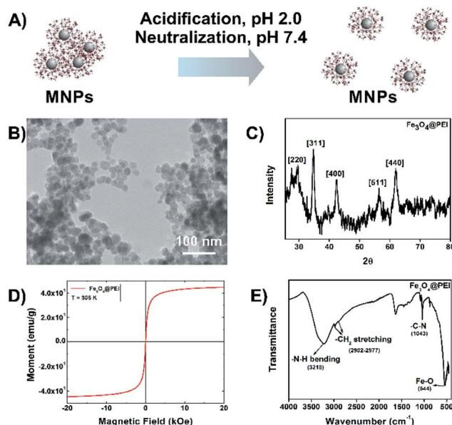
Fig. 2 Characterization of the polyethyleneimine (PEI)-coated  $\text{Fe}_3\text{O}_4$  MNPs. (A) Depiction of non-acidified and acidified MNP dispersion. The MNPs were analyzed by (B) TEM, (C) XRD, (D) VSM, and (E) FTIR for morphological and structural investigation and determination of the crystal structure, magnetization, and functional groups, respectively.
