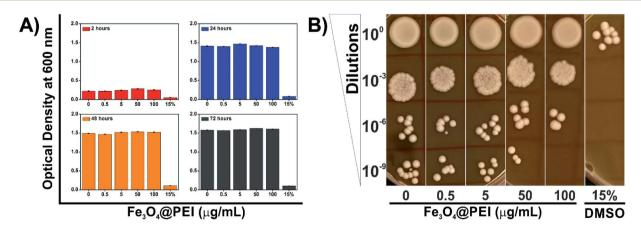
Fig. 4 The toxicity tests for yeast cells. (A) The OD<sub>600</sub> results recorded after 2, 24, 48 and 72 hour incubation of yeast cells in growth media containing different concentrations of Fe<sub>3</sub>O<sub>4</sub>@PEI MNPs and (B) spot test results of samples incubated with MNPs for 72 hours.
