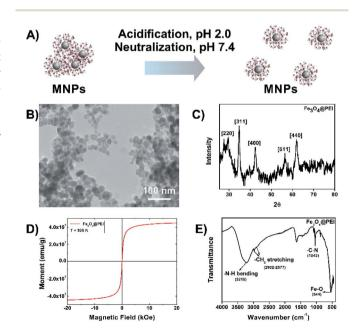
Fig. 2 Characterization of the polyethyleneimine (PEI)-coated  $Fe_3O_4$  MNPs. (A) Depiction of non-acidified and acidified MNP dispersion. The MNPs were analyzed by (B) TEM, (C) XRD, (D) VSM, and (E) FTIR for morphological and structural investigation and determination of the crystal structure, magnetization, and functional groups, respectively.
