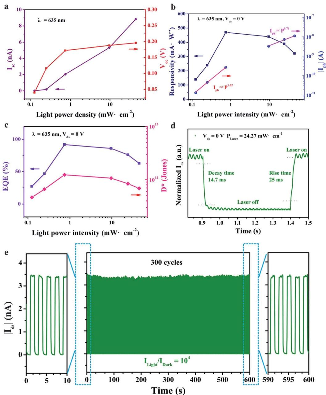
Fig. 4 Self-powered photo-response characteristics of the heterostructure device under 635 nm illumination. (a) The  $V_{oc}$  and  $I_{sc}$  of the device versus illumination power intensity. (b) Photocurrent and  $R_{\lambda}$  varying with incident intensities under 0 V bias. (c) EQE and  $D^*$  as a function of the light power intensity. (d) Rise and decay time of the device under  $24.27 \text{ mW} \cdot \text{cm}^{-2}$ . (e) Photo-response of the photodetector with 300 cycles.
