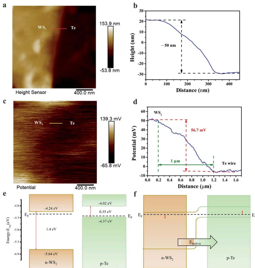
Fig. 2 Characterization and band alignment analysis of the mixed-dimensional heterostructure. (a) AFM image of the WS<sub>2</sub> nanosheet on the Te microwire. (b) The height data of the WS<sub>2</sub> nanosheet along the scale length of the red line in (a). (c) Spatial potential distribution at the heterostructure interface. (d) The SPD along the yellow line in (c). (e) The energy band diagram of the Te microwire and WS<sub>2</sub> heterostructure before contact and (f) after contact.
