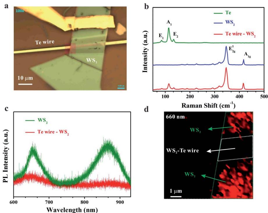
Fig. 1 Raman and PL properties of the heterostructure. (a) Optical image of the mixed-dimensional device. (b) Raman spectrum of the Te microwire, WS<sub>2</sub> and Te microwire–WS<sub>2</sub>. (c) PL spectrum of WS<sub>2</sub> and Te microwire–WS<sub>2</sub> under 532 nm laser excitation. (d) PL mapping of the WS<sub>2</sub> nanosheet on the Te microwire located from the red rectangular region in (a).
