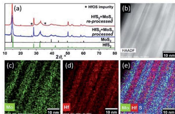
Fig. 2 (a) XRD powder patterns, (b) HAADF-STEM and (c–e) STEM-EDS images of the ball-milled sample of an equimolar mixture of HfS<sub>2</sub> and MoS<sub>2</sub> in a planetary mill for 30 hours and subsequent annealing at 1000 °C for 72 hours, followed by reworking of the material formed using the same processing protocol. XRD patterns of HfS<sub>2</sub> and MoS<sub>2</sub> are shown as references. Bragg peaks of {HfOS} impurity are indicated by asterisks.
