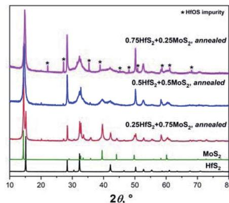
Fig. 3 The XRD patterns of different mixtures of HfS<sub>2</sub> and MoS<sub>2</sub> ball milled in a planetary mill for 30 hours and subsequent annealing at 1000 °C for 72 hours. XRD patterns of starting materials HfS<sub>2</sub> and MoS<sub>2</sub> are shown as references. The Bragg peaks of an oxysulfide impurity (HfOS) are indicated by asterisks.
