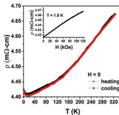
Fig. 7 Electrical resistivity of W<sub>0.4</sub>Mo<sub>0.4</sub>Ta<sub>0.2</sub>S<sub>2</sub> as a function of temperature, measured at heating (black triangle), and cooling (red solid circle) in the absence of magnetic field. Inset shows resistivity as a function of the magnetic field up to 120 kOe at  $T = 1.8$  K.
